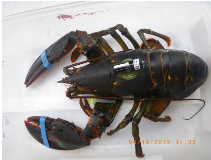
Figure 18. American lobster fitted with a VEMCO V13 acoustic tracking transmitter, and conventional numbered disc tag attached by cable tie above the knuckle.
