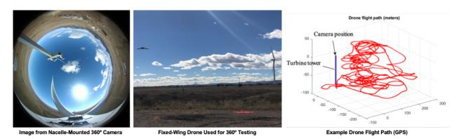
**Figure 17.** Sample image from nacelle-mounted 360° 4K camera (left); fixed-wing drone used for programmed flights and 360° capture (middle); and, GPS recording of drone flight relative to the wind turbine and camera postion (right).
