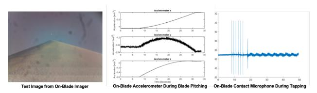
**Figure 19.** Initial validation of on-blade collision detection modules includes remote testing of all sensor subsystems; on-blade image r for down-blade image capture, on-blade IMU (accelerometer and gyrometer), and on-blade contact microphone. All three on-blade modules were validated following installation prior to structured data collection.
