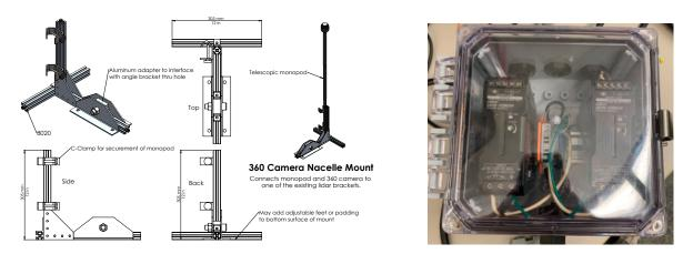
**Figure 14.** (left) Additional custom fixturing was designed and fabricated for mounting 360° camera on the nacelle. (right) Custom DC-DC power conversion assembly for powering on-blade modules from the turbine hub.
