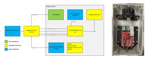
**Figure 10.** (left) Annotated block diagram of second and final version of collision detection system electronics module following first round of on-blade testing to increase local compute power and improve sample synchronization for IMU and contact microphone data streams. (right) Final system in mounted in custom modified enclosure.
