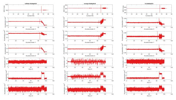
**Figure 23.** Typical data recorded from on-blade multi-sensor modules, with blades pitching from 85° to 0°; pitching begins at approximately 85s, and the impulse visible just prior to this is the mechanical pitching lock being opening at the blade hub.
