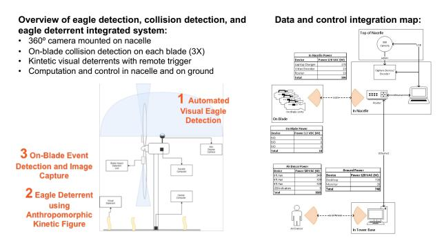
**Figure 13.** (left) Intended location of detection, deterrent, and collision detection system components on an installed wind turbine. (right) Network diagram including wired and wireless connections among subsystems for control and data acquisition across the integrated system.
