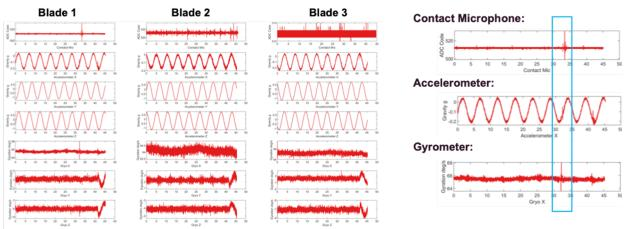
Example Synchronized Recording of Multi-Sensor Data from All Blades
