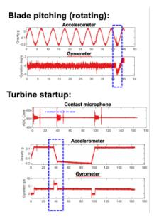
Figure 32. Annotations of typical non-collision turbine and blade actions visible from on-blade sensors, including blade rotation, blade pitching, and turbine startup.
