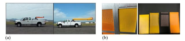
**Figure 6.** (a) Maximum wind velocity testing for visual deterrents Deployment at 55 mph (orange,  $\sim$ 25 m/s) and 45 mph (yellow,  $\sim$ 20 m/s) for the 6- and 20-foot variants. (b) Accelerated weather testing (AWT) of deterrent materials compared to common exterior-use waterproof-breathable fabric (orange) and tarp (yellow) materials; post-AWT samples at right.
