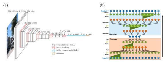
**Figure 4** (a) Illustration of the deep convolutional neural network (CNN) used for extracting a 1000- dimensional deep-feature vector from every video frame. (b) Temporal convolutional neural network (TCNN). Input to the TCNN, X, are deep-feature vectors extracted from each video frame. Output of the TCNN, Y, are class labels assigned to every video frame.
