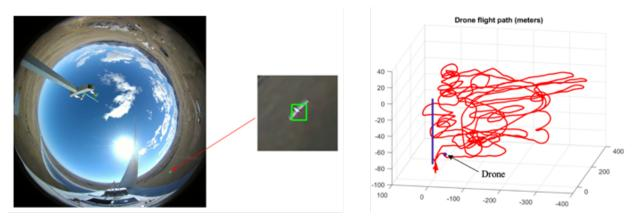
**Figure 18.** Sample image from nacelle-mounted 360° 4K camera (left); zoom in of fixed-wing drone in 360° camera frame with automatic bounding box based on motion detection (middle); and, GPS recording of drone flight relative to the wind turbine and camera postion (right).
