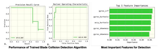
**Figure 34.** Performance of trained collision detection classifier on recorded multi-sensor turbine data collected during NREL-NWTC field testing, including precision and recall and the receiver operation characteristic (ROC); top five features (for driving classification) can be extracted from the forest-based model.
