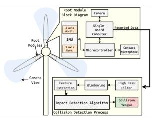
**Figure 8.** High-level block diagram of on-blade collision detection system with automated image capture of colliding objects.
