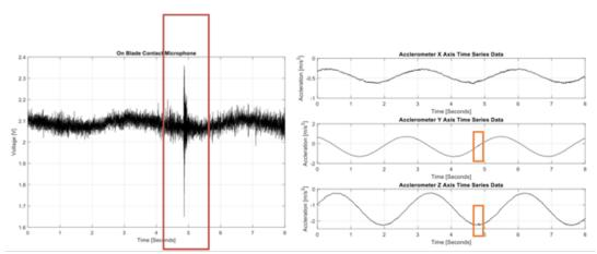
Figure 21. Blade strike by surrogate projectile (tennis ball) recorded using the on-blade sensor module.
