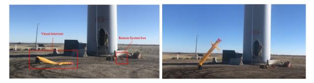
**Figure 16.** Installation and testing of visual deterrent near the base of the 1.5MW wind turbine. The deterrent is activated by an artificial stimulus; in practice, this would be triggered by the eagle detection system (Task 1.00) if eagles were detected in the 360° camera video stream from the nacelle roof.
