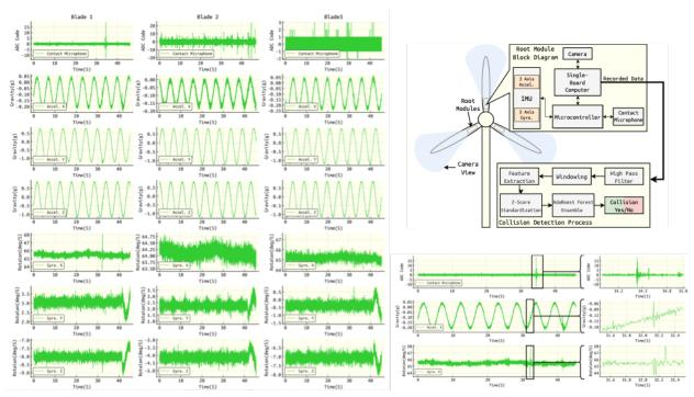
**Figure 33.** Three-blade multi-sensor data (accelerometer, gyrometer, contact microphone) is used as input to train a collision detection classifier algorithm for automated blade-strike collision detection.
