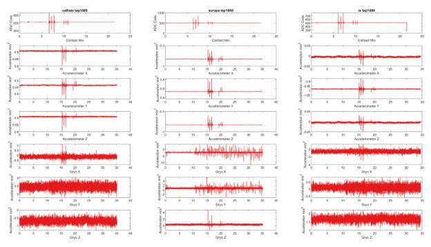
Figure 24. Typical data recorded from tapping on one of the blades (middle column), with the resulting vibrations seen across sensors (accelerometer, contact microphone, gyrometer) and across all blades.
