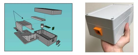
**Figure 11.** (left) Exploded view of the mechanical housing for BID system and corresponding electrical components. (right) External view of assembles BID module in modified IP67-rated enclosure.
