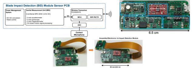
**Figure 9.** (top) Custom multi-sensor module printed circuit board (PCB) integrates accelerometer, gyrometer, contact microphone readout, and power management into a small circuit board for integration into on-blade system. (bottom) Custom sensor PCB connects to small single-board computer and CMOS imager for complete, wireless system.
