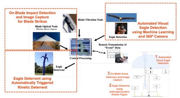
**Figure 1** Overview of integrated system for visual detection of wild eagles, deterrence using a visual kinetic deterrent system, and on-blade sensor and imaging system for automated collision detection and blade strike imaging. The combined system was tested both in parts and as a complete integrated system across multiple fields tests, including testing on operational wind turbines.
