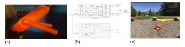
**Figure 5.** (a) A 6ft visual deterrent undergoing initial testing in the OSU wind tunnel; (b) a simple electrical system for power and remote activation of visual deterrents; and, (c) initial testing of the visual deterrent system.
