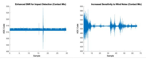
**Figure 25.** SNR is improved over the prior system (left); increased sensitivity also picks up more wind noise while mounted on the blade, so future installations will include a wind cover (Section 3.3).
