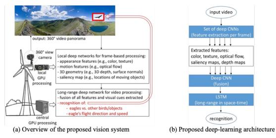
**Figure 2** A  $360^{\circ}$  camera is used to capture a panoramic video. Video processing consists of two stages: feature extraction identifies important visual cues from every frame, and the results of this local processing are fused over long-range time intervals for eagle detection and trajectory estimation. The local and central video processing will be specified as a cascade of deep convolutional neural networks (CNN).
