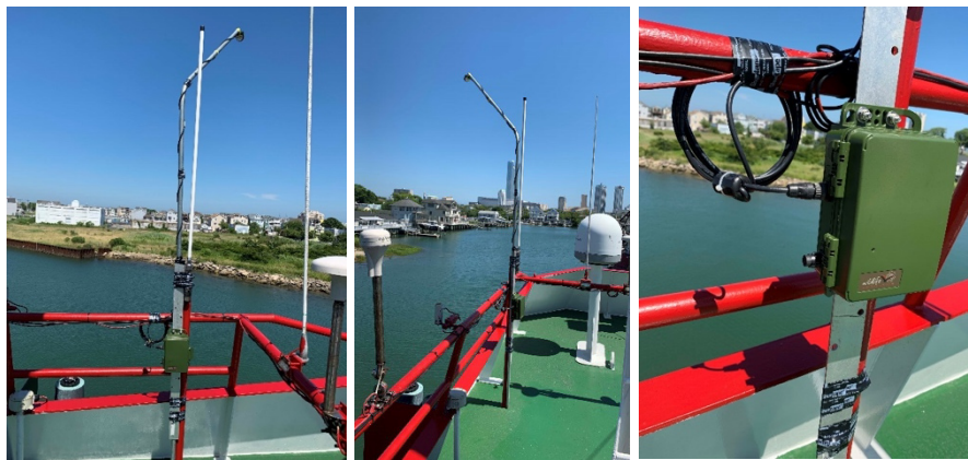
Figure 1. Placement of the bat detector on the survey vessel in 2021.
