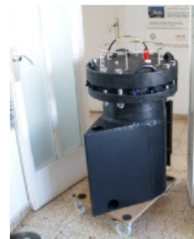
Figure 8: Sonobuoy for marine mammals and underwater noise monitoring.
