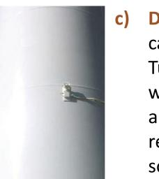
**DTBird® Collision Control Module: HD** cameras survey 360° around the Wind Turbine, detecting birds in real-time while storing videos and data. Potential and accidental bird collisions can be recorded and checked in videos with sound through Online access
