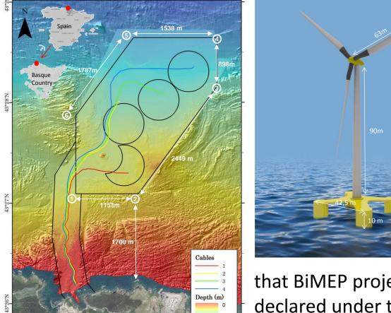
Recent developments have promoted the interest of BiMEP facilities for the testing and demonstration of offshore wind developments as well, allowing the installation of a maximum of 2 offshore floating wind mills of 5 MW each (physical dimensions showed in the picture on the left). Consequently, new and different environmental impacts from the original projects are expected. Among others, an impact over seabirds was foreseen taking into account
