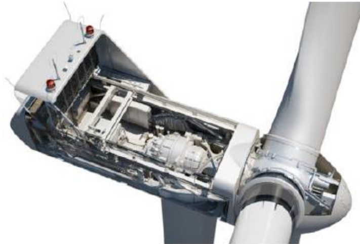
Figure 13. Nacelle and interior components (gear box, main shaft, generator, and control systems).
