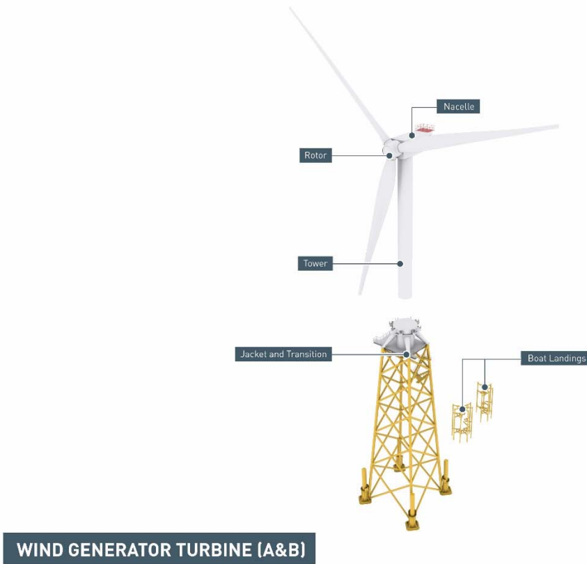
Figure 3.9: Beatrice Wind Turbines Schematic Showing Exploded View
