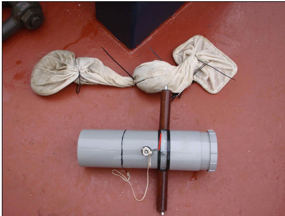
Picture 3. Pitch pipe used to collect sediment for sampling of benthos in the scour holes.
