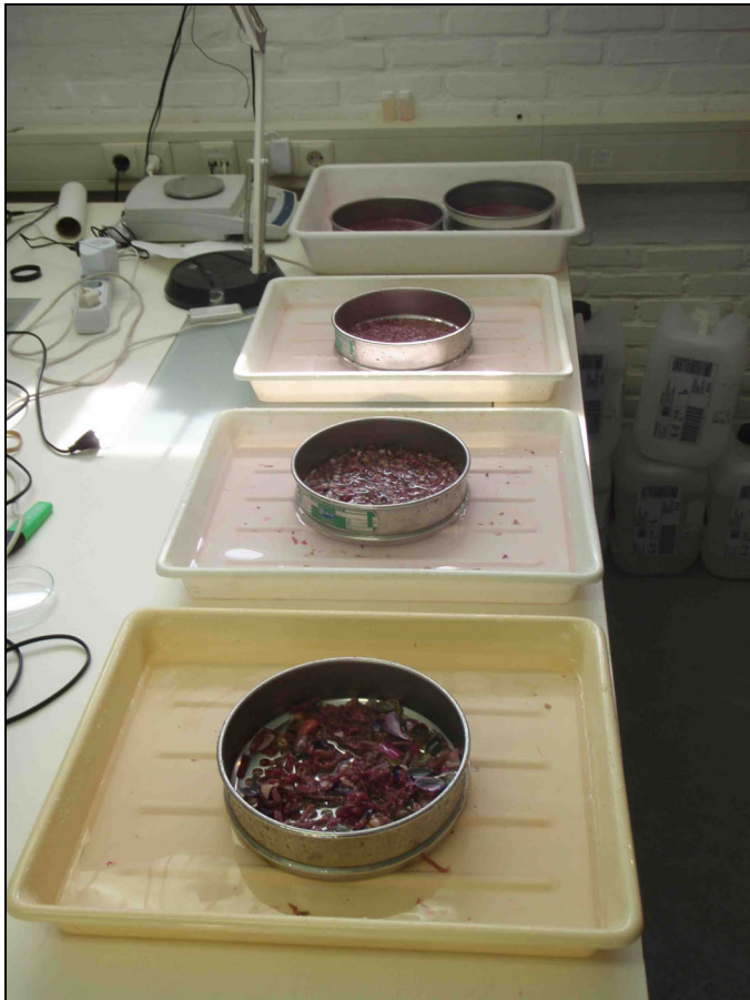
Picture 4. Staining the samples with rose bengal and washing them over a set of nested sieves.
