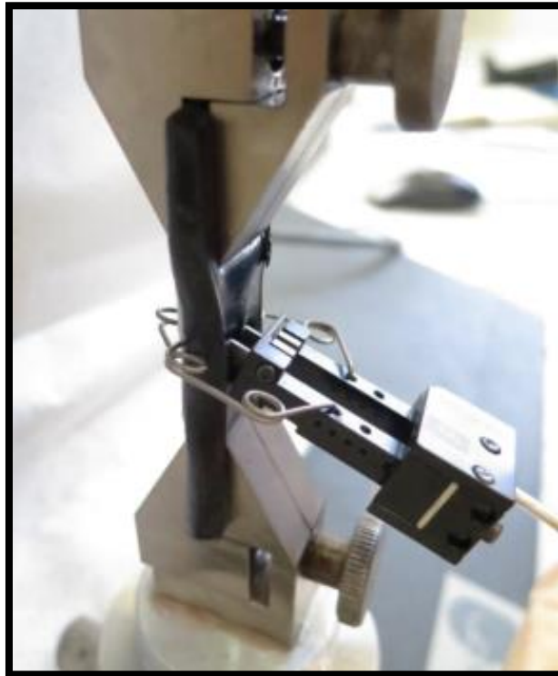
Figure C. 15. The figure shows the MTS with a sample of neonate epidermal tissue within its clamps and an extensometer attached to the sample to measure lateral strain through the test.
