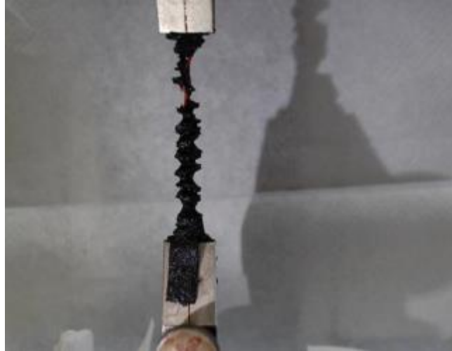
Figure C. 61. Juvenile Skin Rectangular specimen after testing. An example of a thin layer of skin sloughing off can be seen on the bottom clamp. This is a sign of the degradation of the juvenile skin tissue and often happened during tensile testing.
