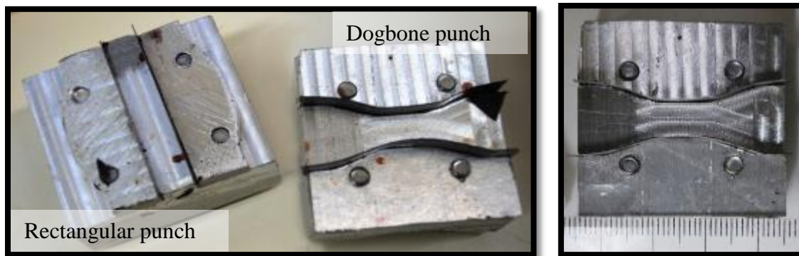
Figure C. 6. Dogbone and rectangular tissue punches are shown above. Samples prepared with the rectangular punch were 40 mm long and 7 mm wide. Those prepared with the dogbone punch were 40 mm long and were 15 mm wide at the top and bottom and 7 mm wide in the narrower middle section.
