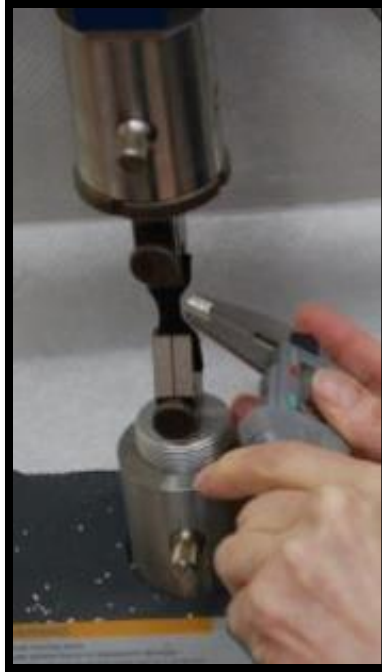
Figure C. 12 Following loading of the test specimen its thickness was measured to the nearest 0.001 mm as shown above using a digital caliper.. The sample thickness was entered into the MTS software program at the beginning of a test.
