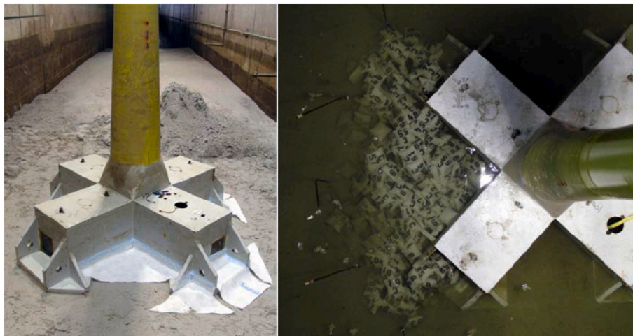
Fig. 14. – Scour protection model of a STRABAG foundation using geotextile containers (Wilms et al., 2012).
