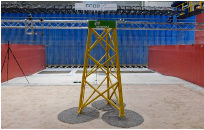
Fig. 10. - Scour protection for a model of the East Anglia One 3-leg jacket (Sarmiento et al., 2021).
