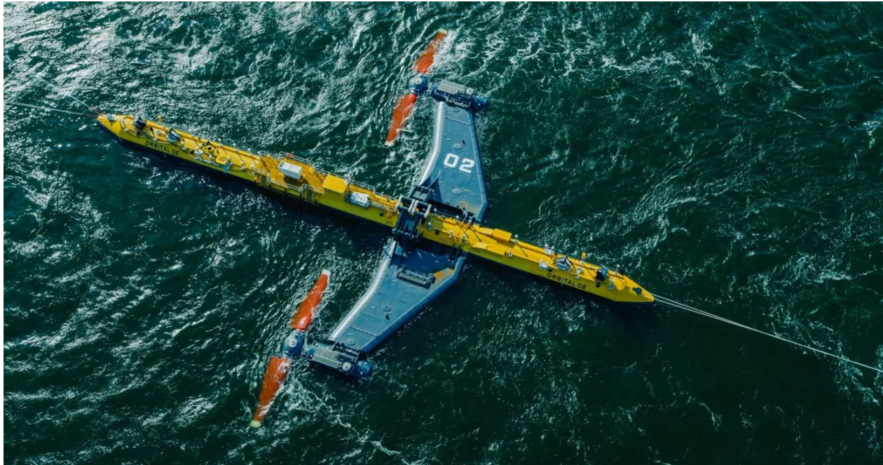
Figure 1. Orbital Marine Technology O2 floating tidal turbine, deployed at the European Marine Energy Center in Orkney, United Kingdom.
