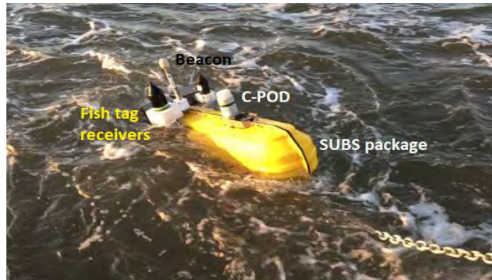
Figure 5: Recently deployed SUBS package containing two fish tag receivers, a beacon from MetOcean Telematics, and C-POD.
