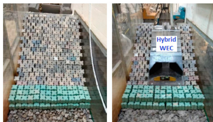
Figure 8. Photographic record of integrated hybrid WEC in a breakwater, 2D physical model without WEC on the left and with WEC on the right.
