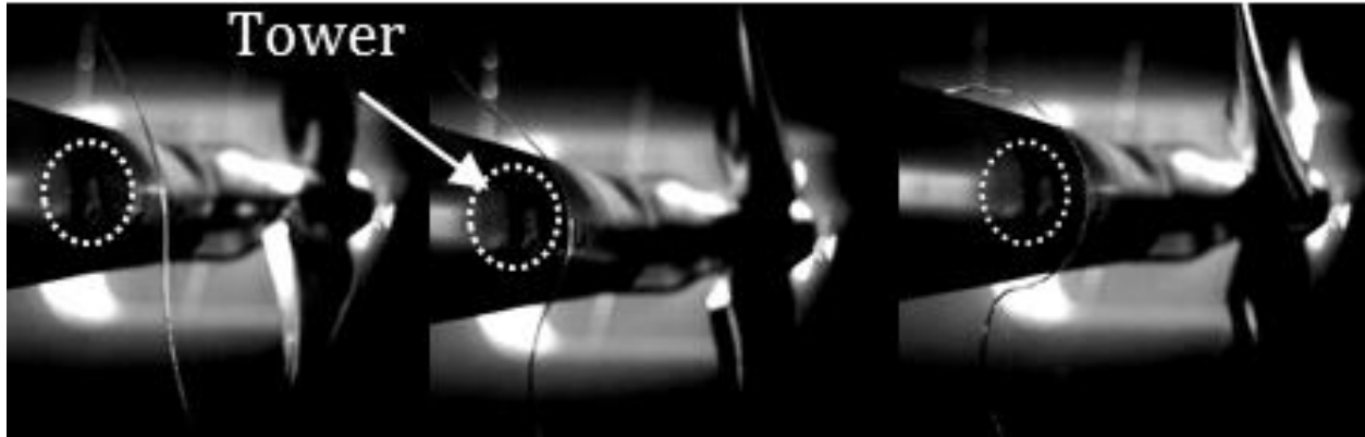
Figure 32. High speed video frames showing tip vortex – tower interaction.
