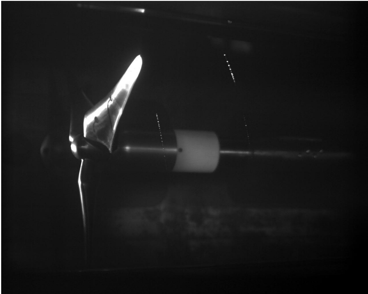
Figure 21. Photograph from Test 3488 of intermittent tip vortex cavitation inception downstream of the Sandia rotor, 4 m/s, 531 rpm, TSR=4, \sigma = 38.7 .
