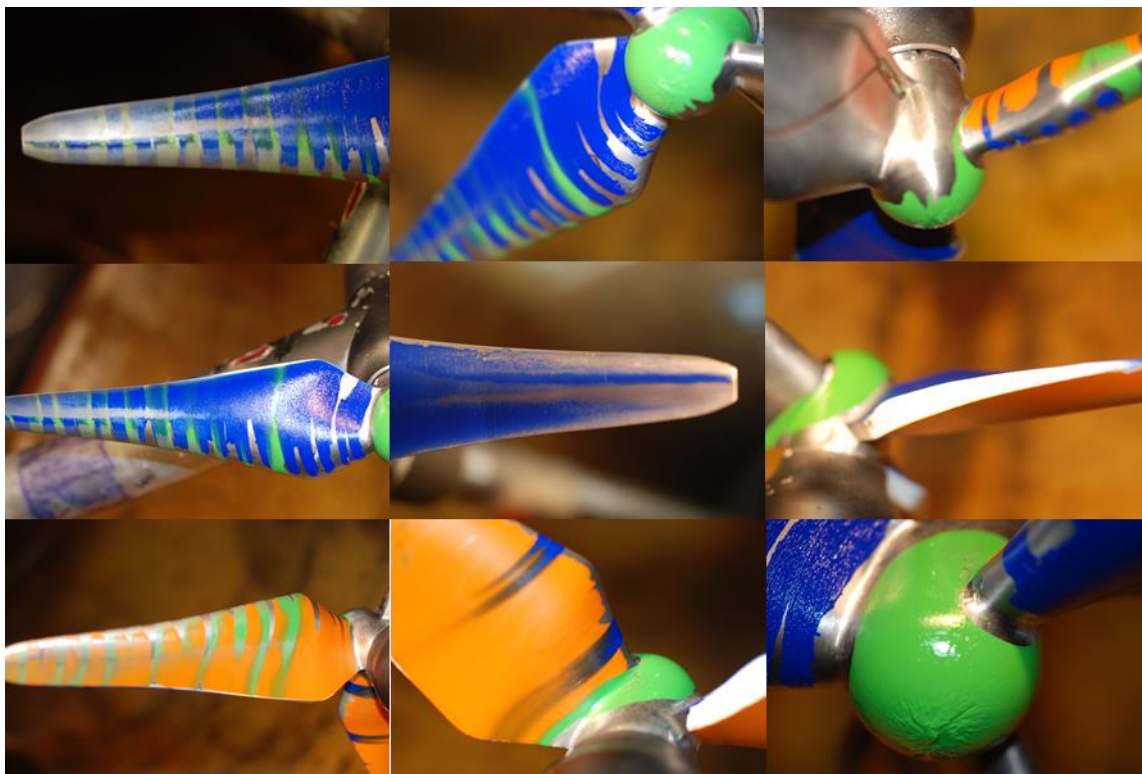
Figure 61. Representative Paint flow features on the model rotor after testing at V_x = 5 m/s and TSR = 4 .
