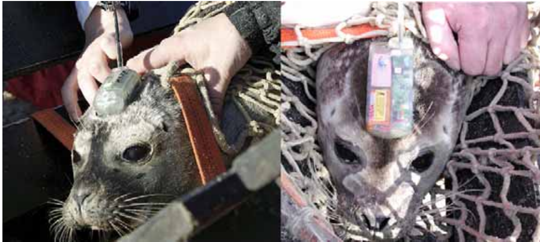
Figure 18. Wildlife Computers SPOT4 (left) and SDR-T16 (right) satellite transmitter mounted on the head of two harbour seals. Antenna faces backwards and electronics and batteries are visible through the translucent plastic moulding. Photos S. Tougaard.
