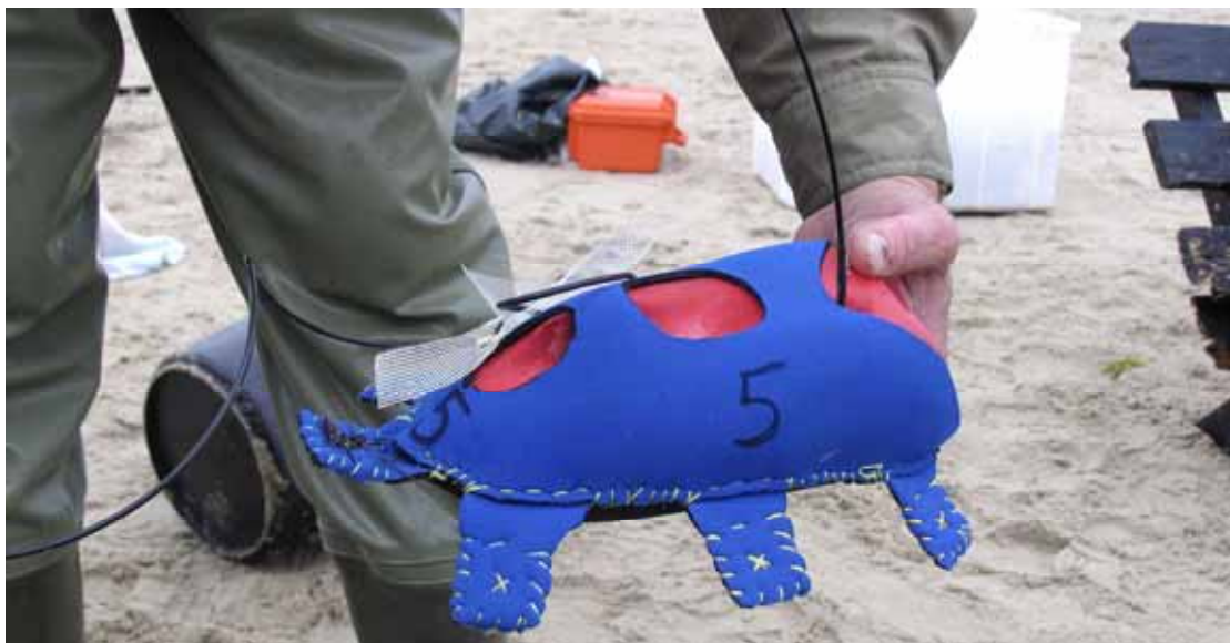
Figure 19. Datalogger ready to be deployed. The red hard foam flotation which contains all electronics is placed inside a neoprene “backpack”, which is glued to the back of the animal at seven points along the edge. To the left is the cable to the IMASEN-device, which is mounted on the head of the animal. Antenna in the rear end of logger (right) belongs to the integral Argos transmitter. Photo: S. Tougaard.
