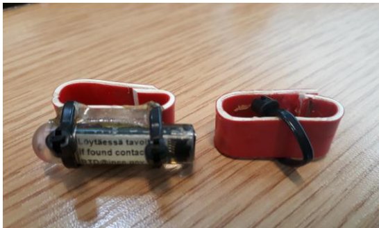
Figure 2. Two darvic rings retrieved in Summer 2019 from divers tagged in Summer 2018. The left ring has a TDR tag still correctly mounted on it; the TDR and one of the cable ties was lost from the right ring.
