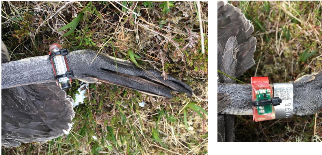
Figure 1. Time depth recorder (TDR) tag (left) and geolocator (GLS) tag (right) mounted on red darvic rings and attached to red-throated diver legs. GLS tags were put on the same leg as the metal ID ring. Photo: Sue O'Brien.
