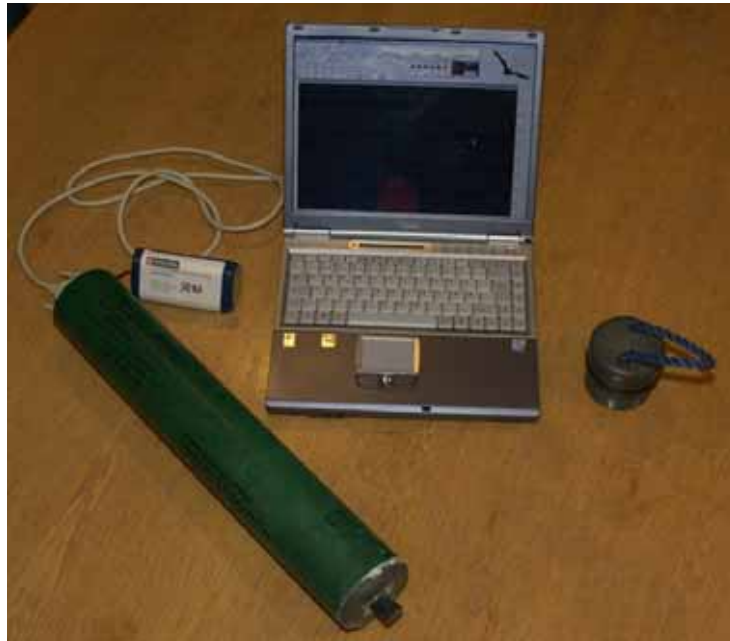
Figure 20 An open T-POD connected to a computer. The hydrophone can be seen as a small attachment in the lower end of the T-POD. A prefabricated 6xD-cell LiIon battery pack is seen behind the T-POD.
