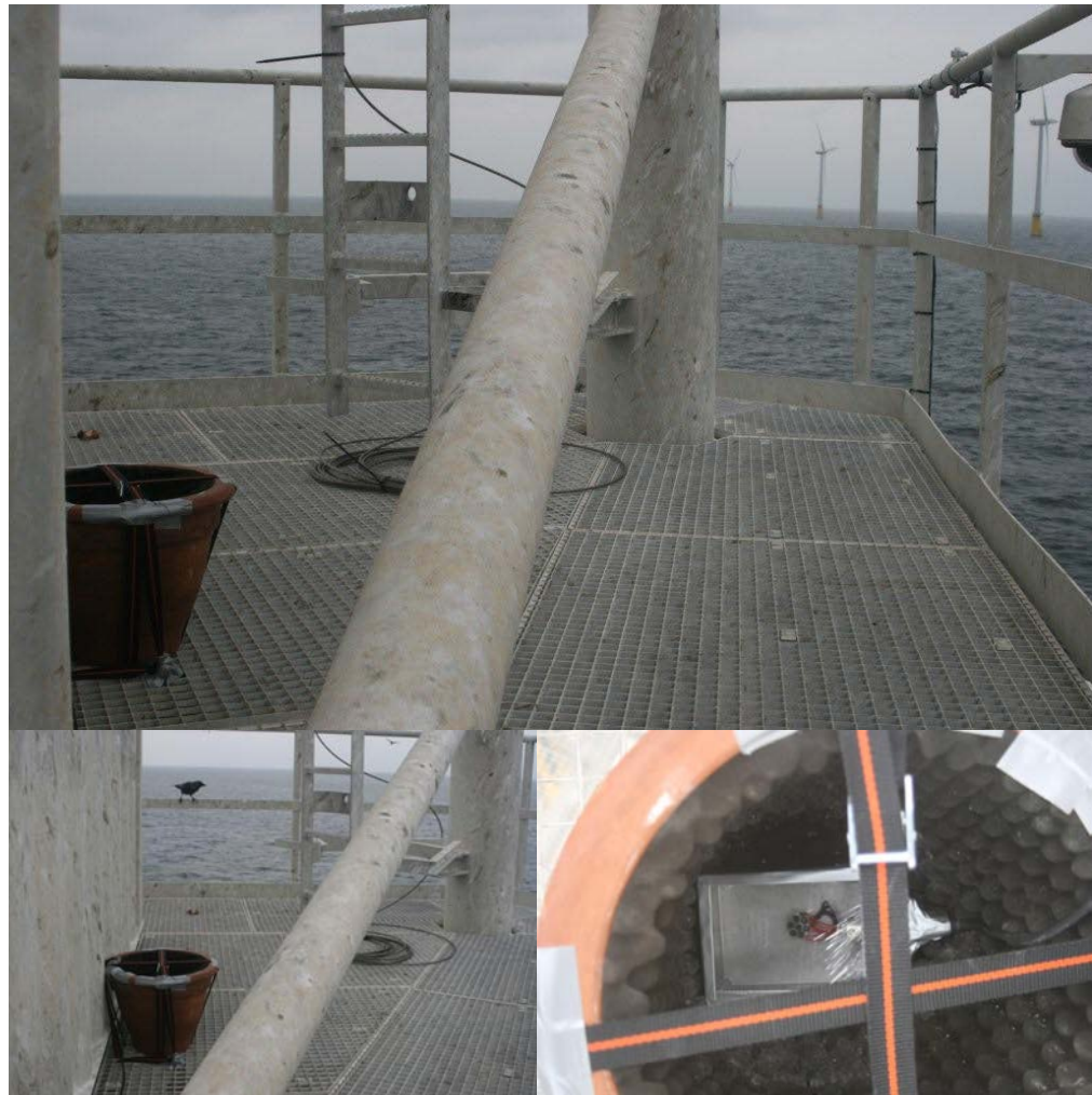
Figure 4.4 The set-up of the outdoor microphone at the metmast. The microphone consisted of 7 Panasonic WM-61 electret microphone elements in a custom made wind- and rain-shield construction. A jackdaw is safeguarding the equipment.
