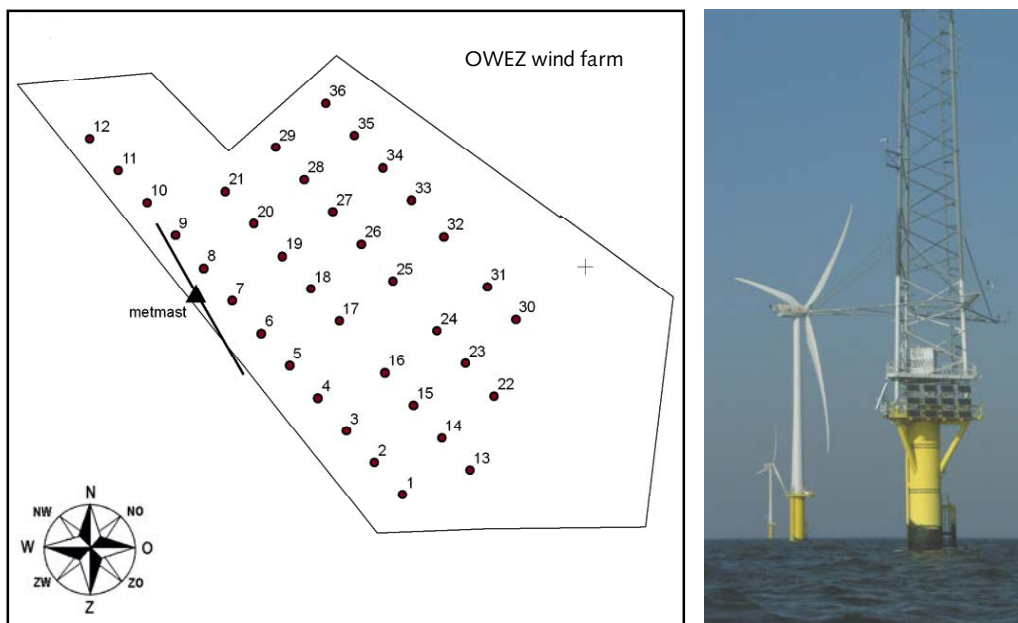
Figure 3.2 Outline of the wind farm with the position of the metmast (triangle) as well as orientation of the vertical radar beam (black line through metmast). The photo shows the metmast from the south and two wind turbines in the back (photo: K. Krijgsveld).
