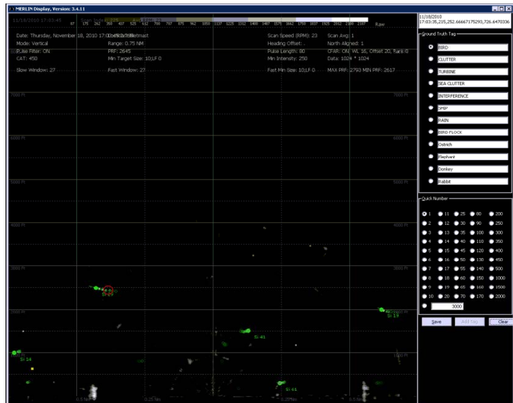
Figure 7.8 Flagging procedure for vertical radar. Echoes that are recorded by Merlin are visible as green closed circles on the Merlin display screen. Each recorded signal remains visible as a green open circle for some time after it has been recorded, leaving a so-called echo-trail. These green circles can be selected with the cursor, and flagged digitally as belonging to e.g., a bird, ship, rain, sea clutter or otherwise. Here, thrushes migrating SW in autumn are flagged as 'birds'. Two turbines are visible as white objects at the bottom of the screen. See fig. 6.10 for a simultaneous view of the horizontal radar.
