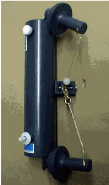
Figure 11: On the left a Niskin sampler. On the right a Chlorophyll a profile with DCM
