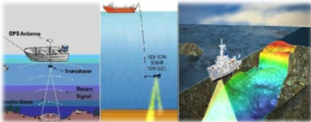
Figure 6: Single beam (left), Side Scan sonar (centre) and Multibeam techniques (right)
