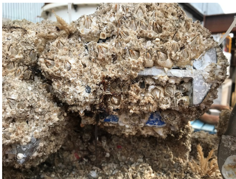
Figure 2. Front-end of a Tritech Gemini sonar unit after approximately 22 months underwater. Extensive biofouling is apparent on the transducers.
