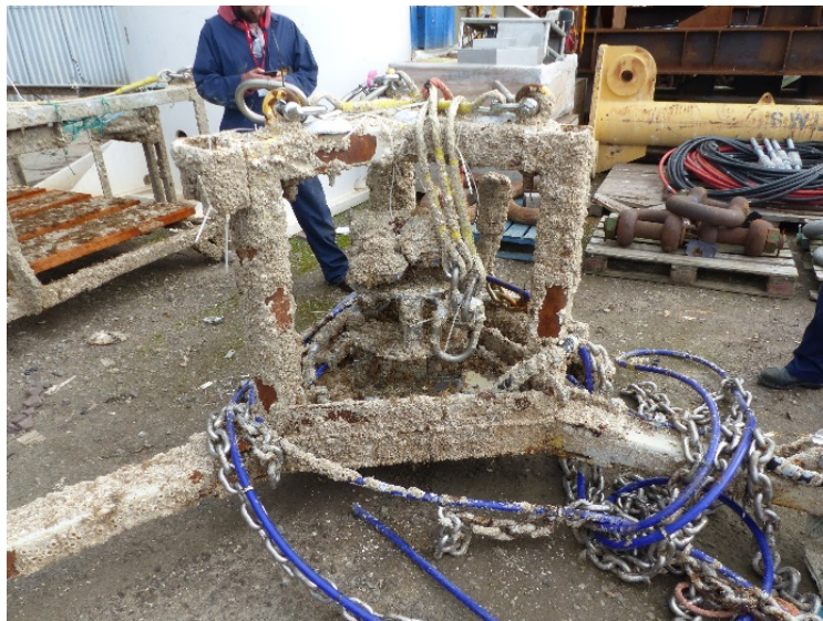
Figure 1. HiCUP at Nigg Energy Park following recovery. Extensive biofouling is apparent.
