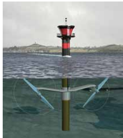
Figure 1-3: Horizontal Axis Turbine - Marine Current Turbines - SeaGen
