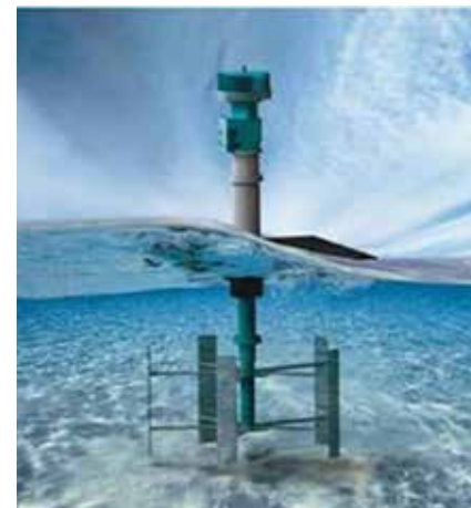
Figure 1-4: Vertical Axis Turbine, New Energy Corporation
