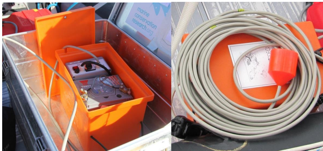
Figure 2.2: Lofitech ADD unit, showing the pulse generator and power source in weatherproof housing (left) and transducer head (right).
