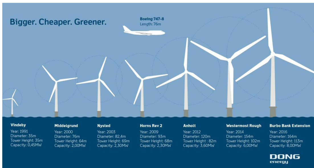
Figure 1.1: Diagrammatic representation of the progress in development of increasingly larger turbines for use in offshore wind farms. Source: humberbusiness.com .
