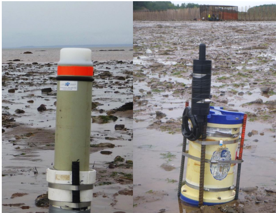
Figure 38: Image of a C-POD (left) and an icListenHF hydrophone (right) and battery pack located at Bramber weir site.
