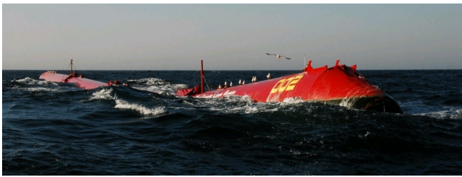
Figure J: Photograph of Pelamis Wave Power device (Source: Pelamis Wave Power)
