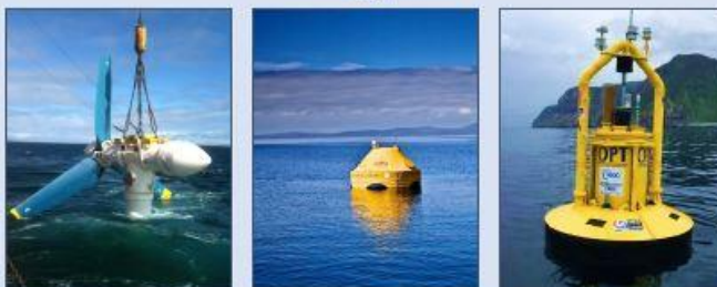
Examples of marine energy devices, including tidal and wave power systems. Pictured examples include (from left to right): SIMEC Atlantis AR1000, CorPower Ocean C3 point absorber, and Ocean Power Technologies PB3.
