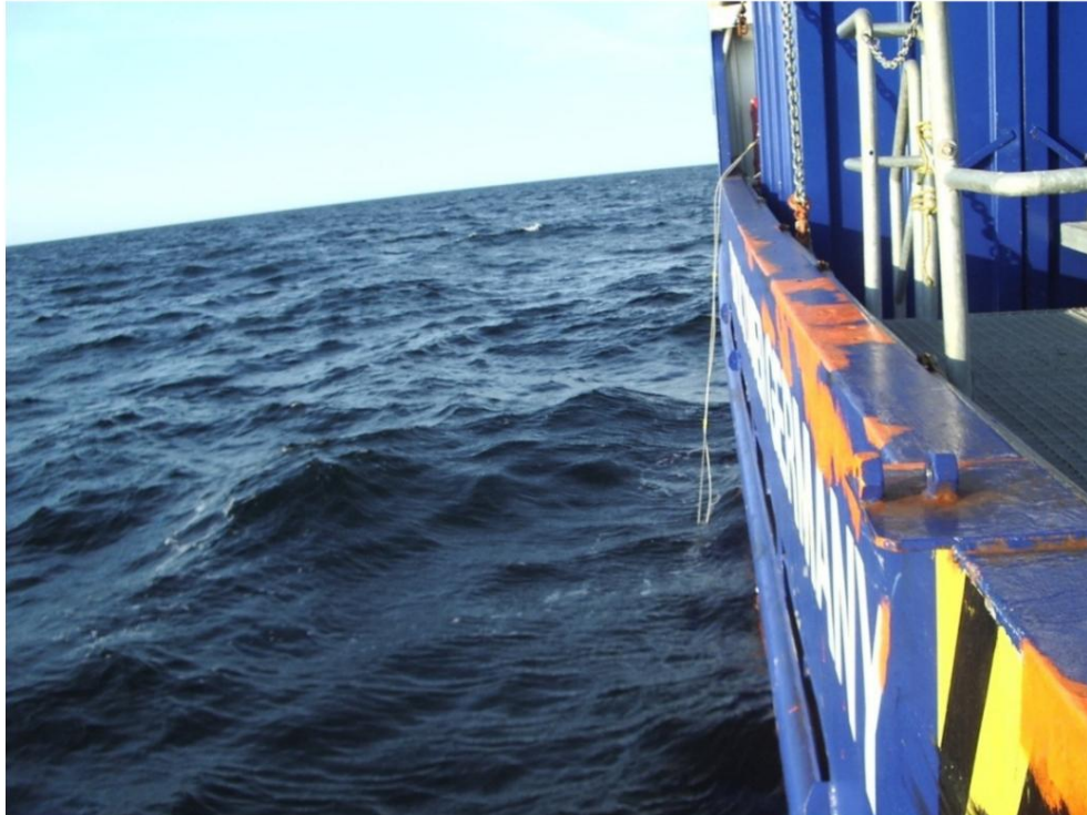
Figure 5-7: Hydrophone cable on the ship's side (DEWI)
