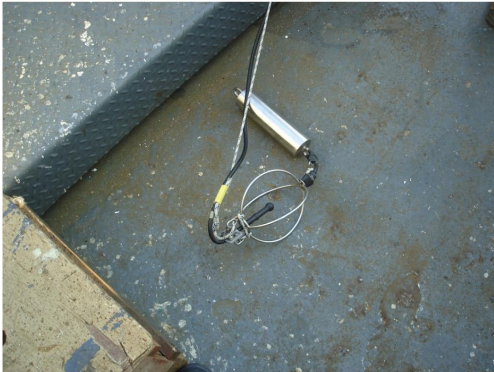
Figure 5-6: Hydrophone with protective cage and weight (DEWI)
