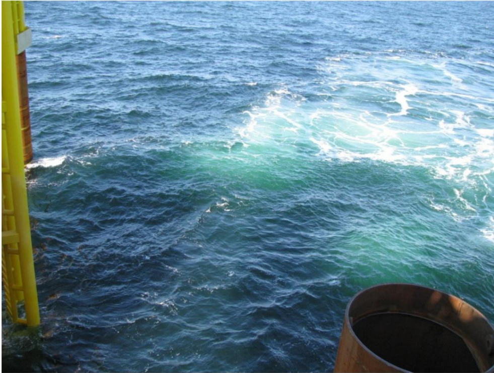
Fig. 5-23: Drift of the bubble curtain at 16:43 (CEST), on the left edge of the picture the northeast pole behind the yellow painted ladder of the tripod, on the lower edge of the picture the Southeast Stake (ISD)
