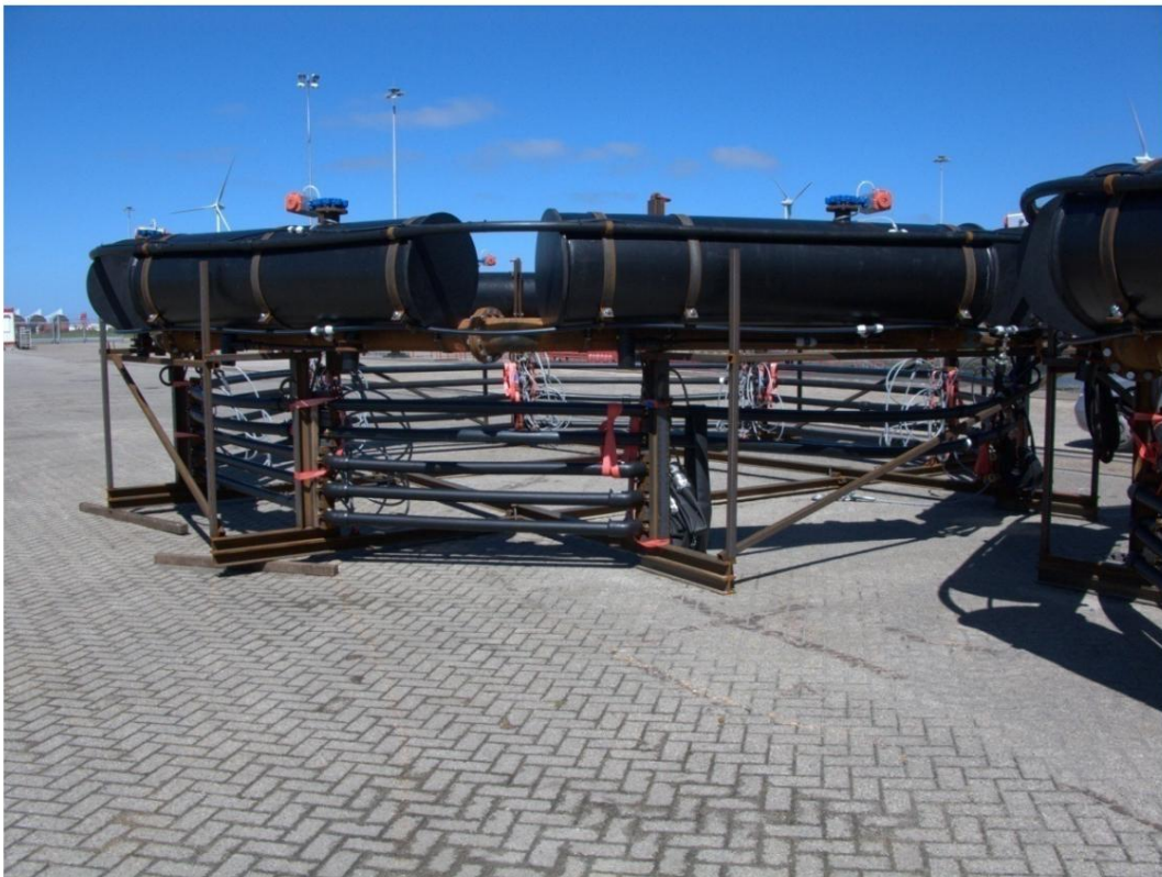
Picture 4-4: Upper bubble curtain on its storage and transport frame
