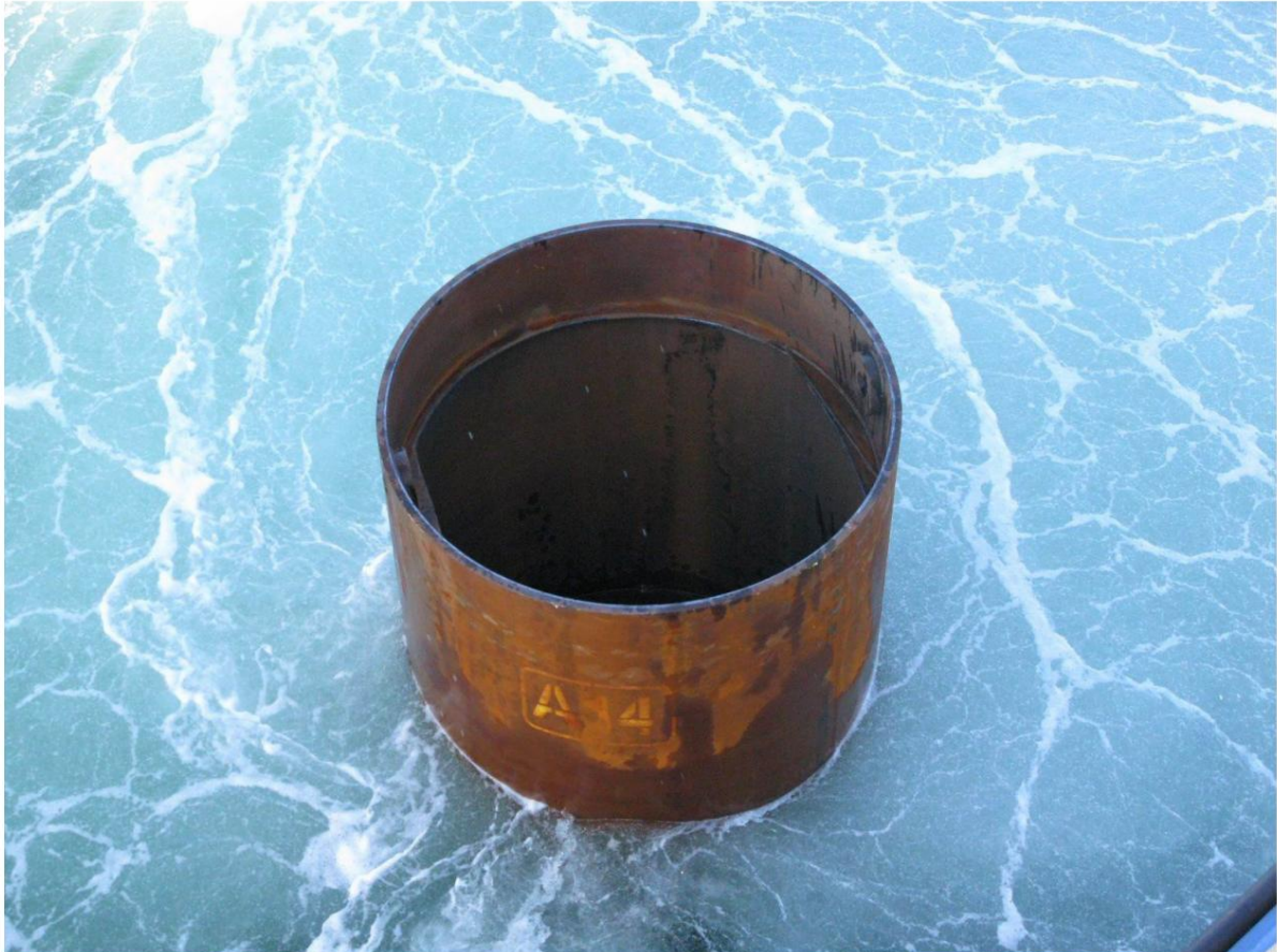
Fig. 4-9: Bubble formation on the water surface at post A14 in the alpha ventus test field
