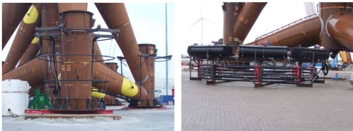
Fig. 2-1 (left:) Lower subsystem of the Bubble Curtain pre-assembled on the AV9, Eemshaven, The Netherlands, (Source: Hydrotechnik Lübeck GmbH); (right:) Upper mobile subsystem of the bubble curtain in the transport frame with buoyancy bodies, Eemshaven, Netherlands (Source: Hydrotechnik Lübeck GmbH)
