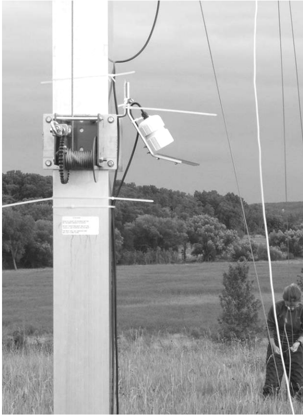
Figure 3. Detector microphone enclosure “Bat Hat” shown mounted at 2m on mobile tower.
