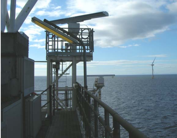
Figure 2. The S-band radar (larger antenna) in position on Beatrice Alpha platform, overlooking the wind turbine site (© University of Aberdeen).
