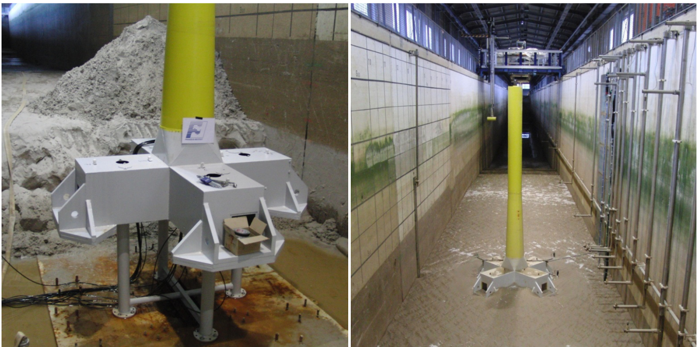
Figure 4-5: Gravity based foundation installation in the GWK wave flume for scour experiments.
