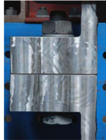
Figure 2-15: left: testing machine for fatigue test under pure bending (Pat.-No. 10 04 258), right: flange segment connection for fatigue test und combined loading; Berger & Schaumann (2008)
