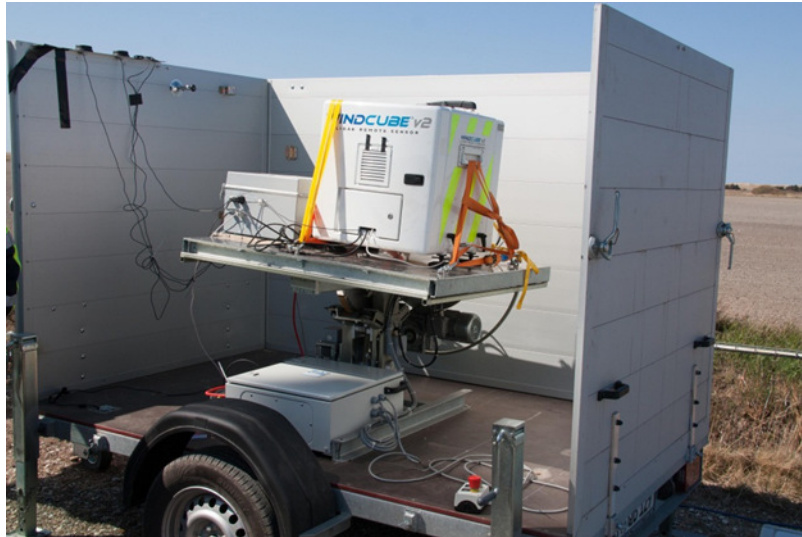
Figure 5-13 A lidar for a floating buoy being tested on a motion platform at Høvsøre.
