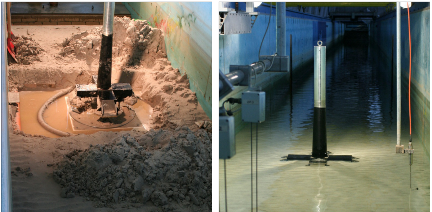
Figure 4-3: Left: Foundation installation in the WKS wave flume with drainage system and lime sand bricks. Right: Foundation during water filling.
