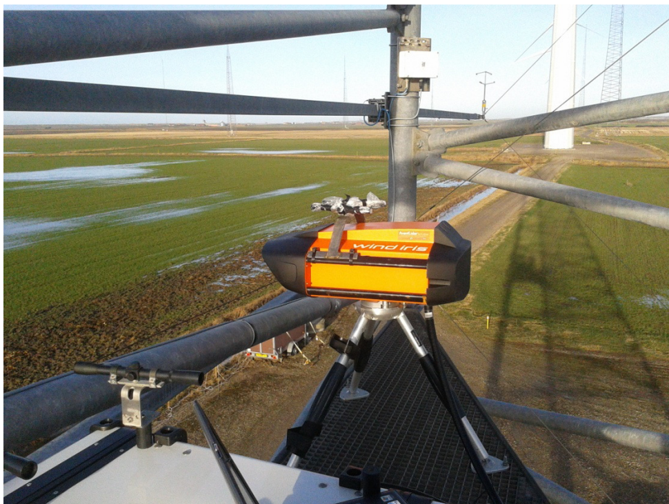
Figure 5-12 A nacelle lidar being calibrated at the Høvsøre test station.
