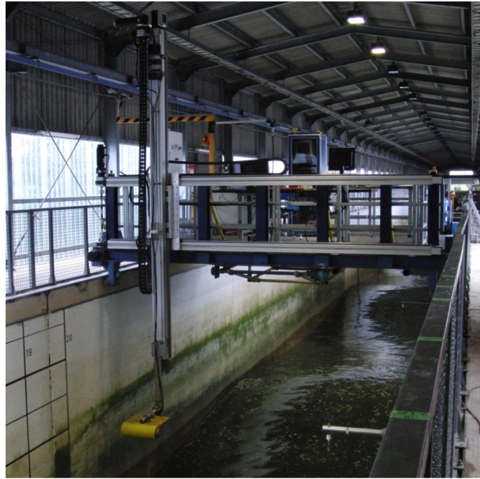
Figure 4-8: Multi-beam echo sounder and positioning platform installation for collection of bed surface profiles during GWK wave flume scour experiments.
