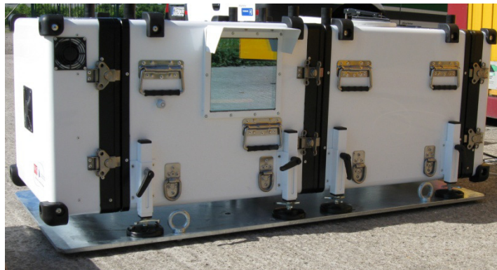
Figure 5-3: SWE lidar scanner based on a commercial pulsed lidar (right hand side) and a self-developed scanner (left hand side)
