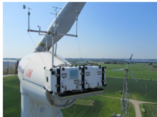
Figure 5-1: Lidar scanner operating at the German offshore test site “Alpha Ventus” (left) [GL-GH],
