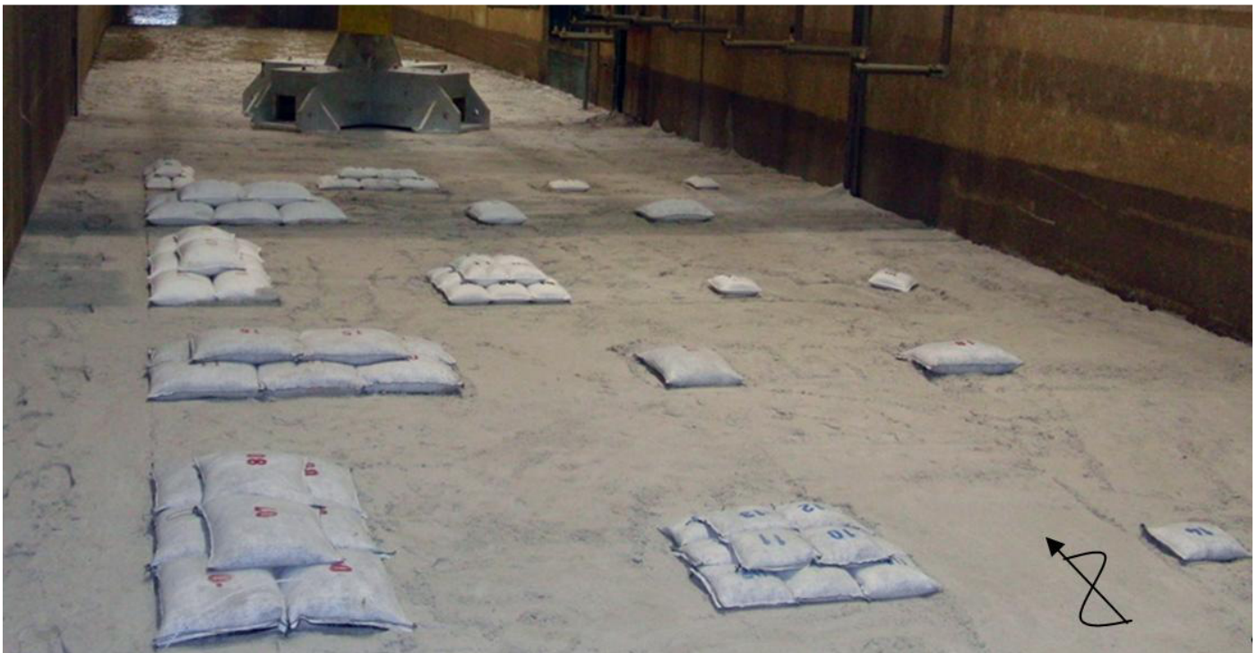
Figure 4-6: Arrangement of sand-filled geotextile containers (before test).
