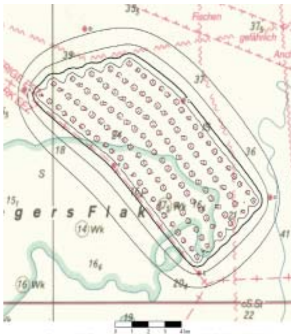
The inner rings around each wind turbine represents 55 dB(A). Thereafter the noise level reduces with 5 dB(A) for each line that surrounds the wind farm.
