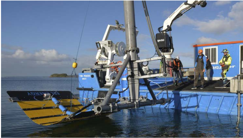
Figure 5. The Eel Energy prototype of biomimetic undulating membrane for tidal energy production (scale 1/6 for a device of 2,5 by 3 m) (source: IFREMER, Eel Energy)
