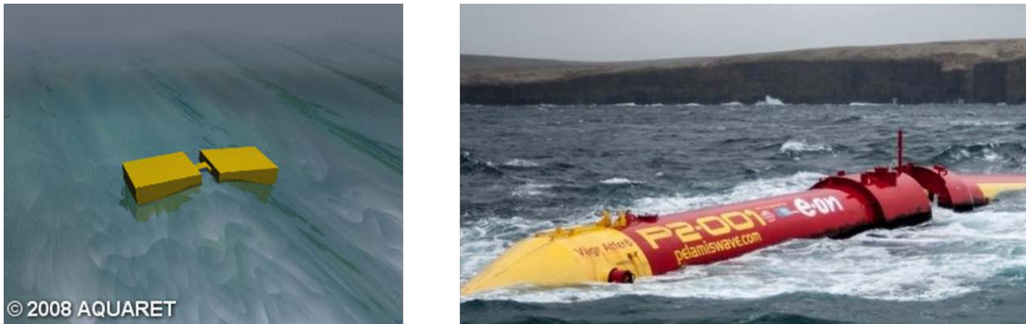
Figure 11. Right Panel: schematic of wave attenuator. Right Panel: the Pelamis wave device at EMEC, Orkney (EMEC 2014).
