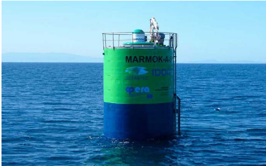
Figure 24a. MARMOK-A-5 device deployed by IDOM at BIMEP after refitting with OPERA innovations.
