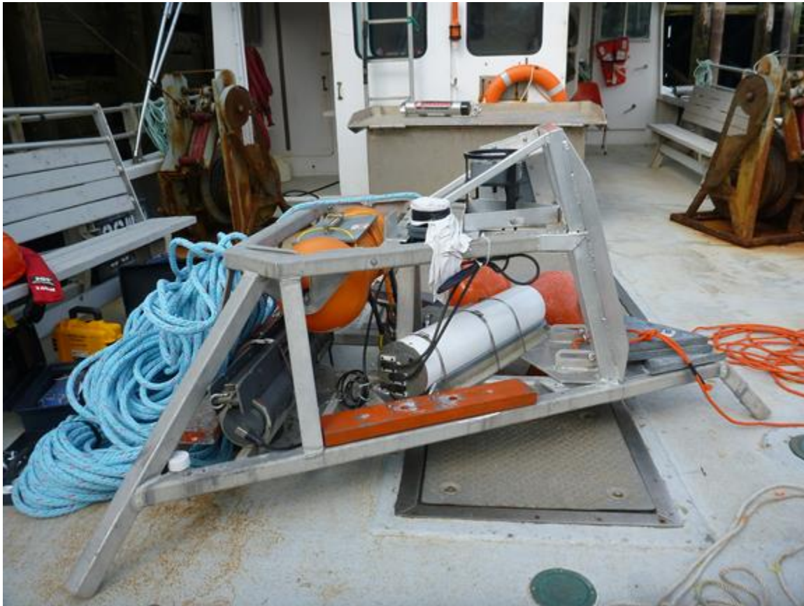
Figure A4-1. The ASL water profiler deployment platform illustrating the positioning of the unit, acoustic release, retrieval dumbbell, and deployment line (blue rope).
