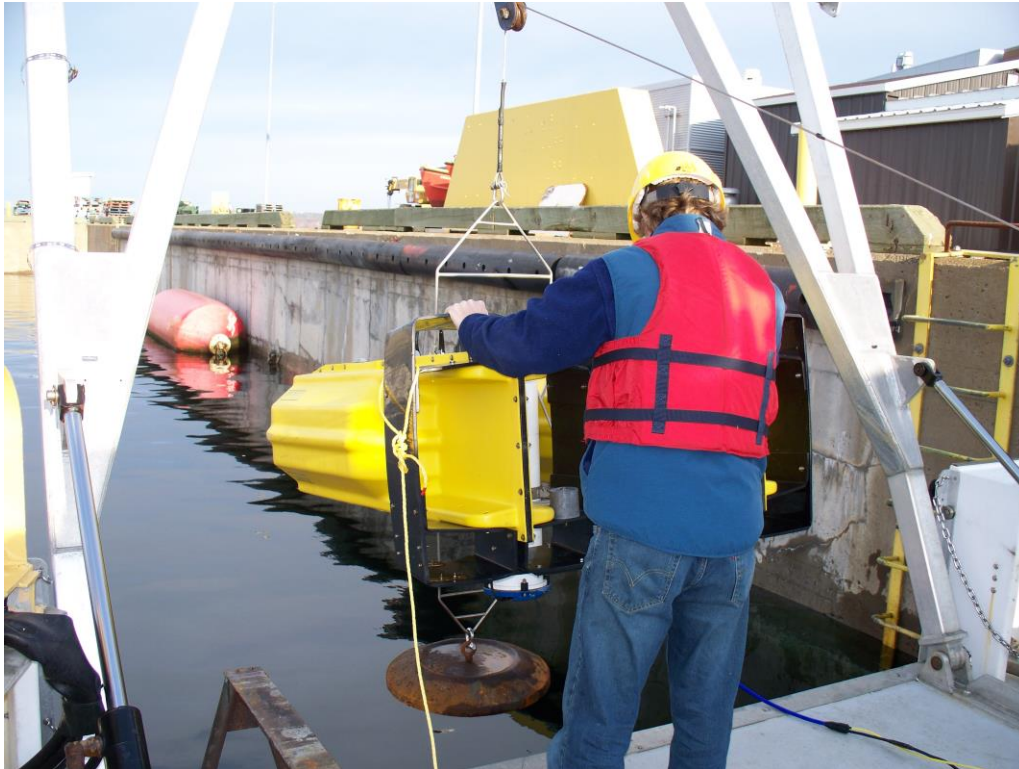
Figure A3-1. Coda Octopus Echoscope II sonar mounted on adjustable-depth flotation package being deployed from SIGMA-T alongside BIO wharf.
