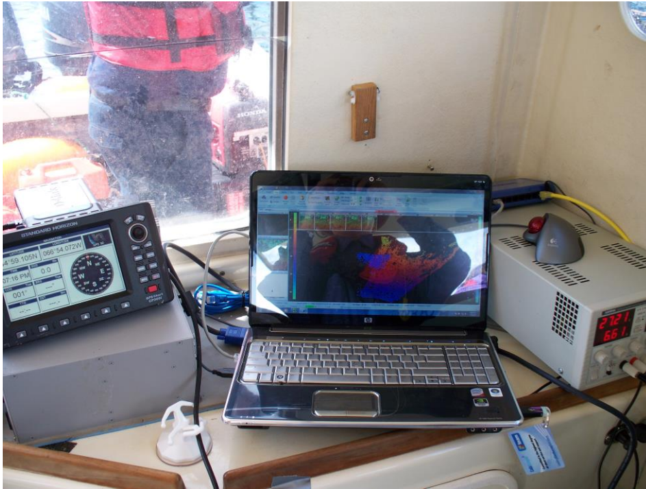
Figure A3-4. Top end control computer for Coda sonar during test in White Island fish weir. Bottom bathymetry is displayed on screen while supply at right provides power to sonar head and DIU.
