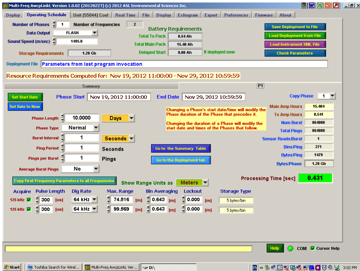
Figure A4-4. ASL software parameter screen showing the settings for the Western Passage deployment.
