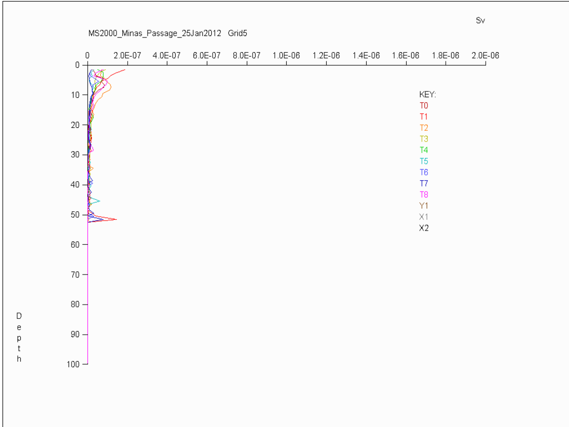
Relative S_v (linear) vs. depth (m) Grid 5, 26 Jan. 2012 Minas Passage survey. Intensive grid lines T0 – T8 only.
