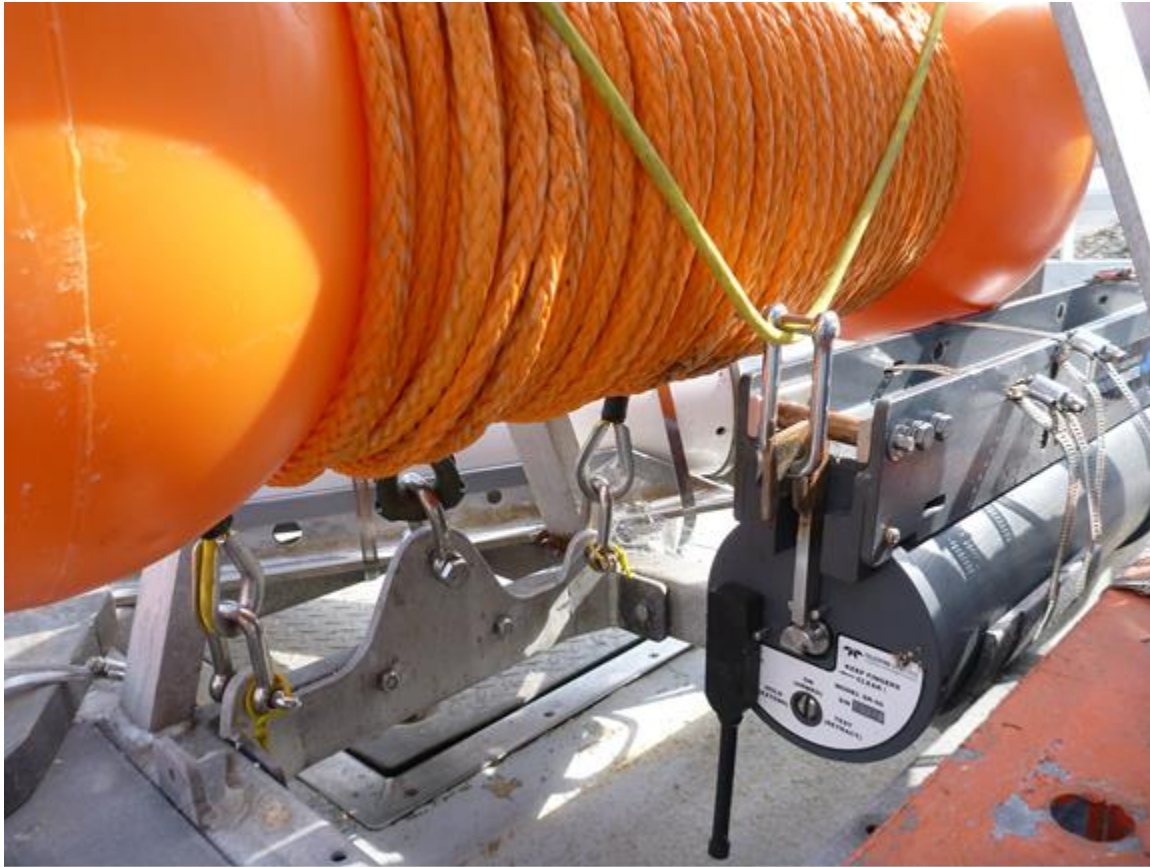
Figure A4-2. Acoustic retrieval mechanism for the ASL deployment platform. The picture illustrates the acoustic release connection to the dumbbell.
