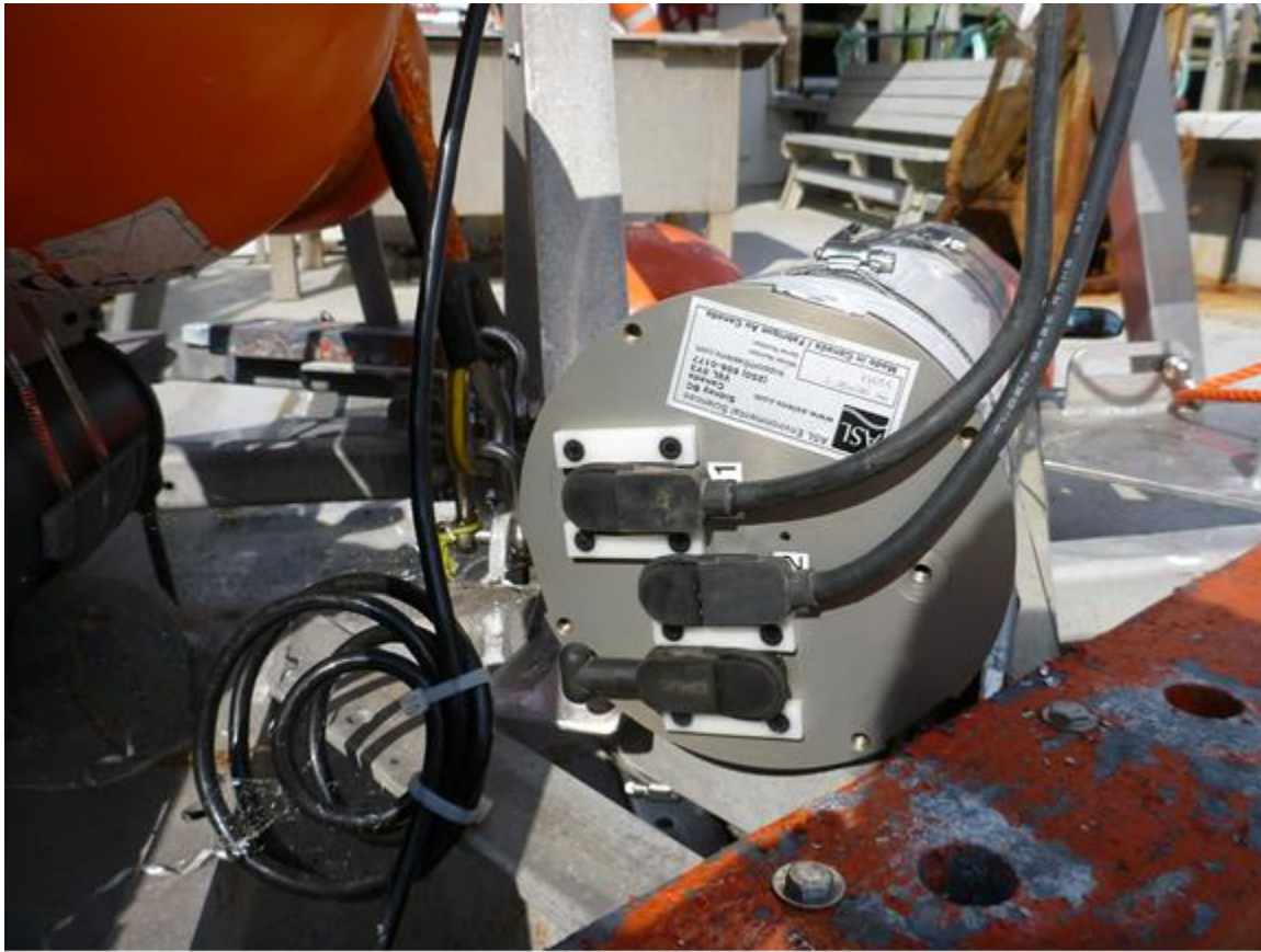
Figure A4-3. Close-up of the ASL water column profiler illustrating the communication port and the transducer connecting cables.
