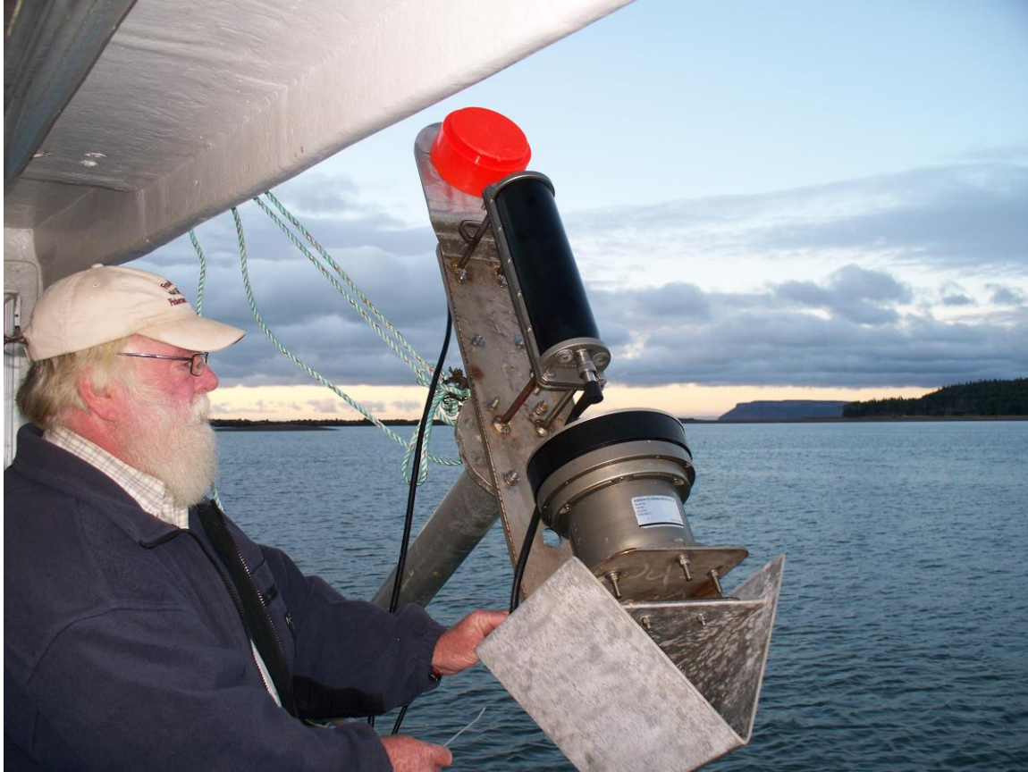
Figure 3. Boom-mounted acoustic transducer package attended by DFO Research Scientist G. Melvin. The orange unit at top is the 120 kHz Simrad EK60 split-beam transducer. Immediately below it lies the 200 kHz Kongsberg-Mesotech MS 2000 narrow beam, linear transmit transducer. Near bottom is the circular arc MS 2000 receive transducer.
