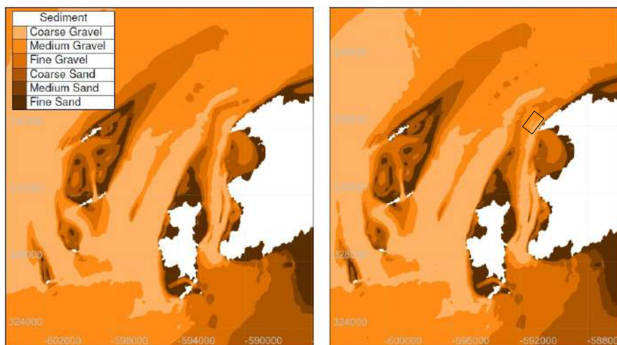
Fig. 2. Estimated sediment maps for no (left) and 9 (right) devices during peak flood (south-north flow).
