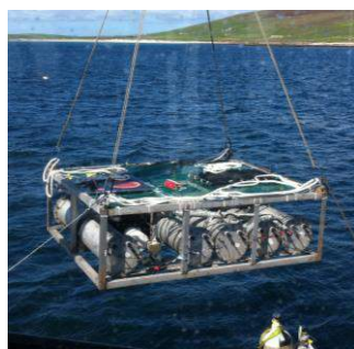
Figure 1. Deployment of the self-contained FLOWBEC platform at EMEC.
