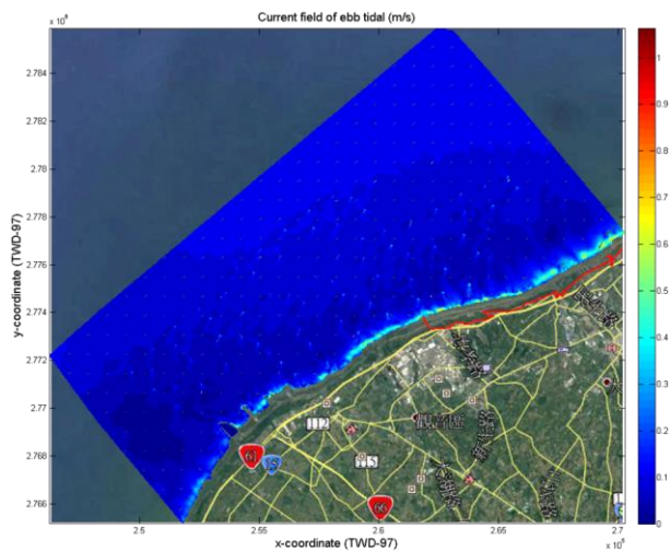
Fig. 22 Current field of ebb tidal during typhoon after set up the wind turbine
