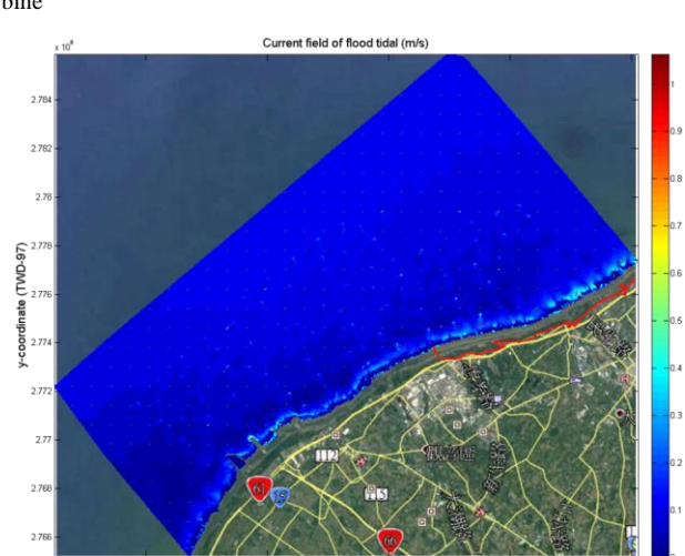
Fig. 21 Current field of flood tidal during typhoon after set up the wind turbine
