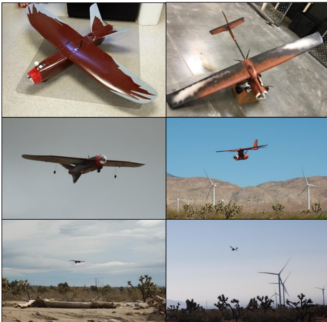
Figure 7. UAV Aircraft Used During the Study to Evaluate the Detection and Deterrent-Triggering Responses of the DTBird System. (a) left = UAV1; (b) right = UAV2.
