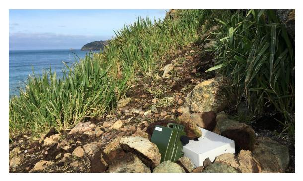
**Figure 6. Passive, digital acoustic recording unit** Scientists use these tools to quantify vocal activity levels and environmental sounds within remote habitats used by seabirds. For example, this technology can be used to study the distribution of seabirds without causing damage to sensitive habitat or disturbing the animals. (Credit: Emma Kelsey, USGS Western Ecological Research Center. Public domain.)
