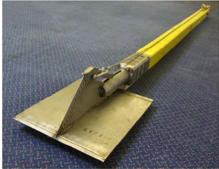
1/10 th scale model of 12m 2 Pennla and 120mT lubricating modular pile
