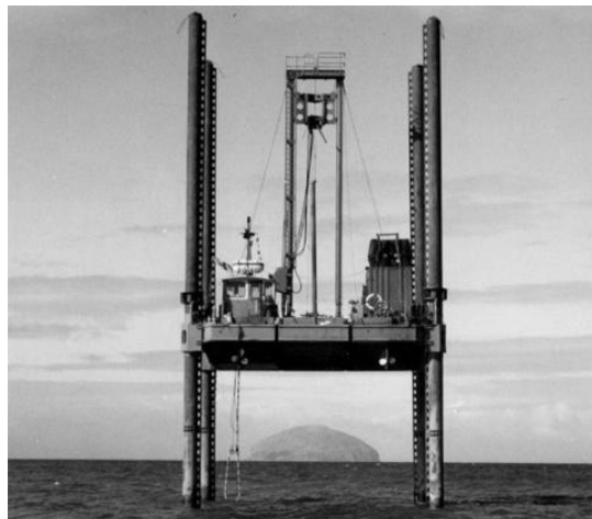
Geotechnical jack-up drill rig
