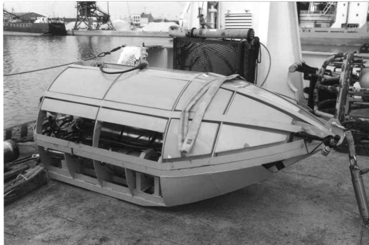
GAMBAS® refraction seismic system – seabed tow sled
