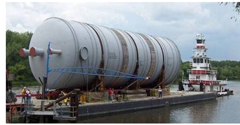
Figure 63 Flat Barge with WEC-Sized device
