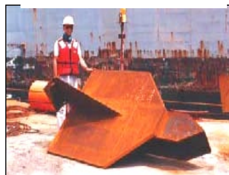
Figure 19 Coral Plate Driven Anchor
