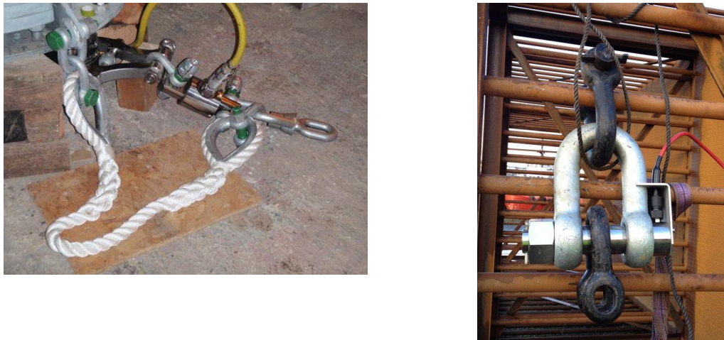
Figure 15 Example of loadcells: a) axial and triaxial loadcells used at SWMTF; b) axial loadcell used on Fred Olsen LifeSaver Bolt 2 device installed at FaBTest
