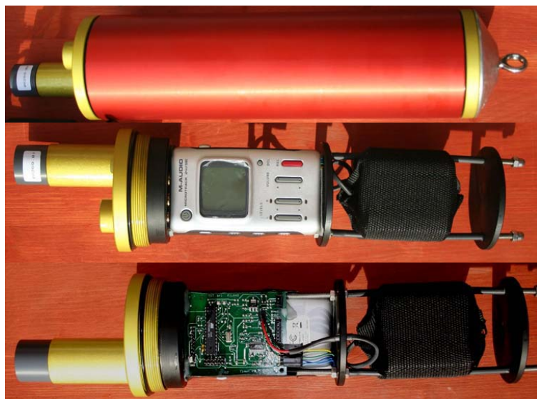
Figure 31. NAUTA’s Programmable Underwater Acoustic Recorder (Registratore Acustico Subacqueo Programmabile, RASP), showing the (top) aluminum housing, (middle) recorder, and (bottom) timer control board.
