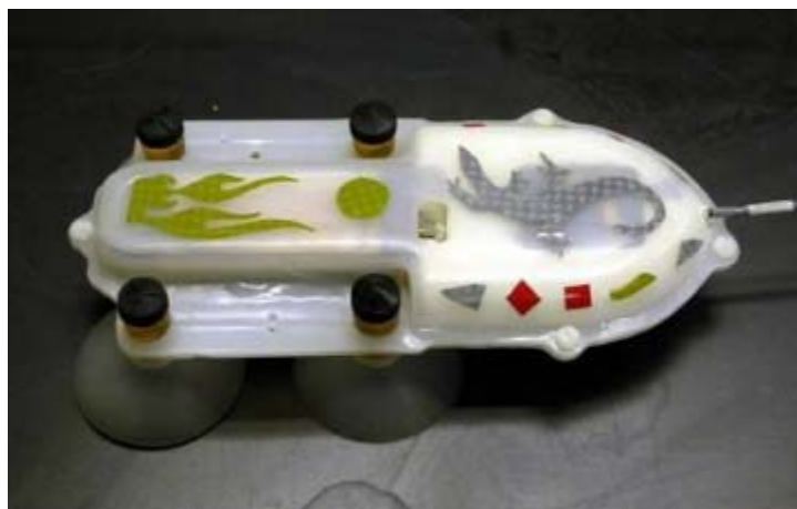
Figure 26. A picture of an assembled Digital Acoustic Recording Tag (DTAG) with casing and suction cups.
