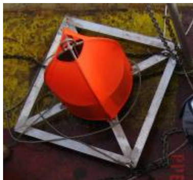
Figure 25. Photograph of a Directional Autonomous Seafloor Acoustic Recorder (DASAR) on deck after retrieval.
