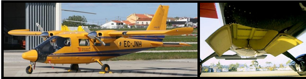
Figure 4–35. Aircraft selected for development of the project scale protocol for offshore high-resolution aerial wildlife imaging surveys: the Vulcanair P68 Observer2 (left) and its belly hatch (right).
