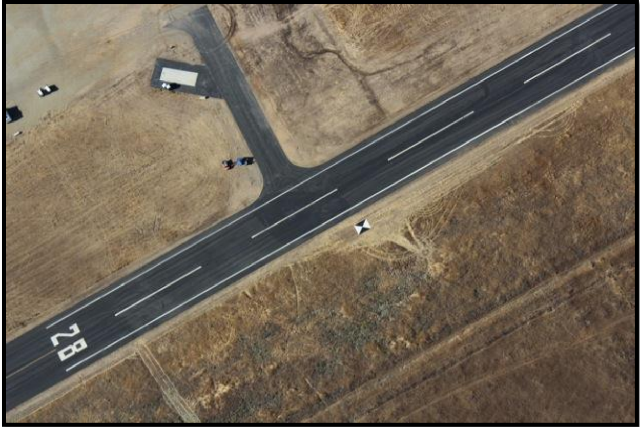
Figure 2–27. Image of the ground surface at Camp Roberts CA, taken during stage 3 flight testing of the UAS-based imaging system, October 2011. Flight altitude = 436 m agl. The black and white image quality evaluation target is visible just below the runway in this image. The dimensions of the target are 457 \times 366 cm.
