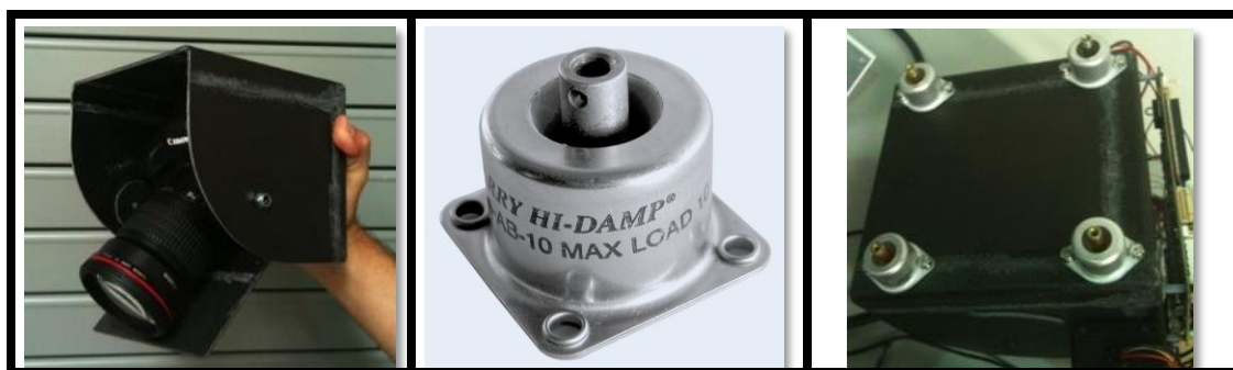
Figure 3–21. Camera and enclosure (left), passive vibration isolator (center), and enclosure with isolators (right) used for UAS-based aerial imaging experiments (see text).
