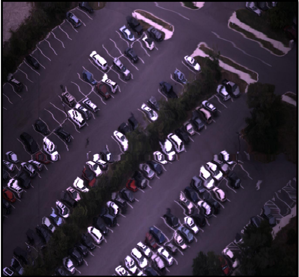
Figure 3–19. Image of a parking lot taken using the line-scan camera on an unstabilized mount (see text) during initial testing flights near Raleigh NC during the first week of May 2011. The waviness in the image illustrates the sensitivity of line-scan cameras to vibrational effects (see text).
