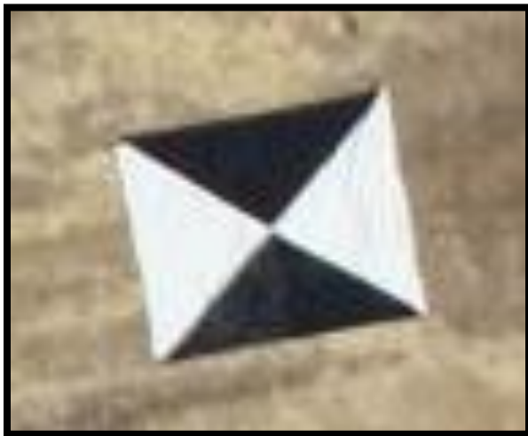
Figure 3–27. Enlargement of a portion of the image from Figure 3–26, showing the calibration object which measured 457 \times 366 cm. The resolution of this image is approximately 2.5 cm.
