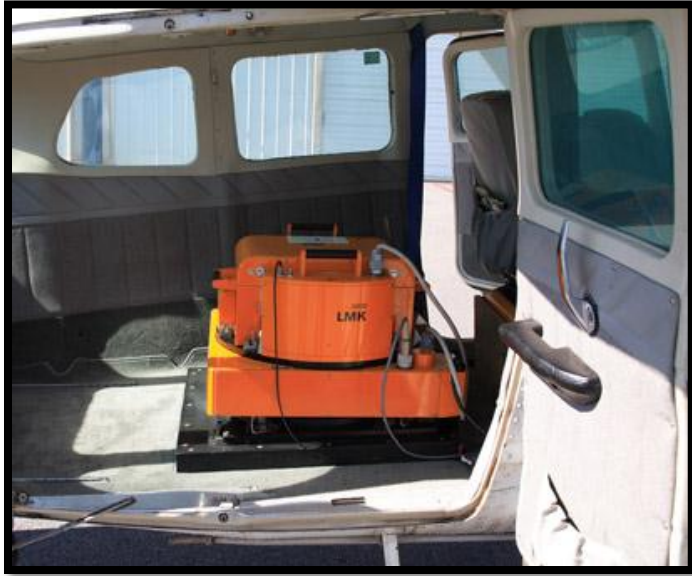
Figure 4–22. Zeiss Jena LMK 2000 mapping camera mounted in a Cessna 206.
