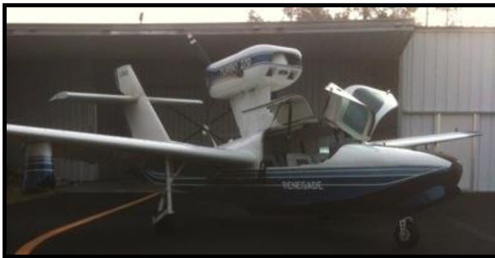
Figure 2–18. Lake Renegade manned aircraft flown over Lake Santa Fe near Gainesville FL during stage 1 flight testing of the imaging system developed for UAS-based aerial high-resolution imaging surveys, September 2011.
