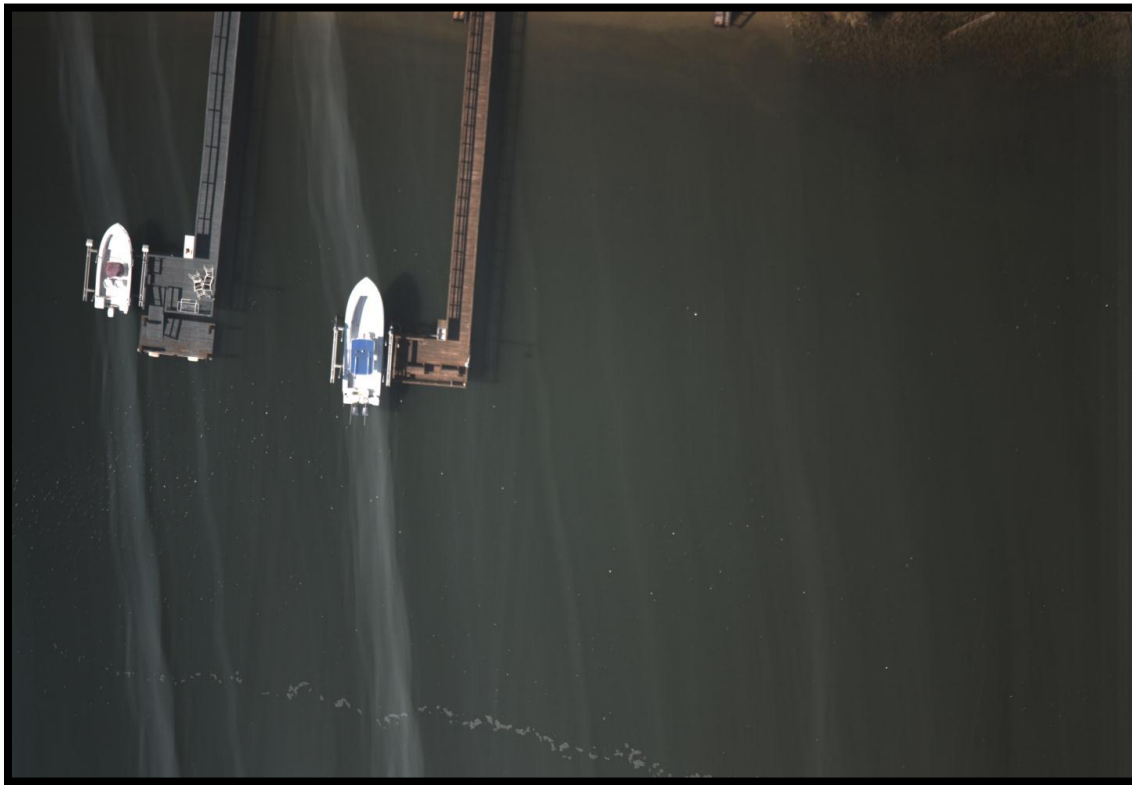
Figure 3–16. Image of boats and docks from aerial imaging experiments conducted 10 to 20 May 2011 offshore of Oak Island NC, showing image smearing effects (whitish vertical streaks in the image). These streaks are an artifact of residual light being let in by the mechanical shutter during digital frame readout and can be eliminated in future applications by using a faster mechanical shutter than was used (see text).
