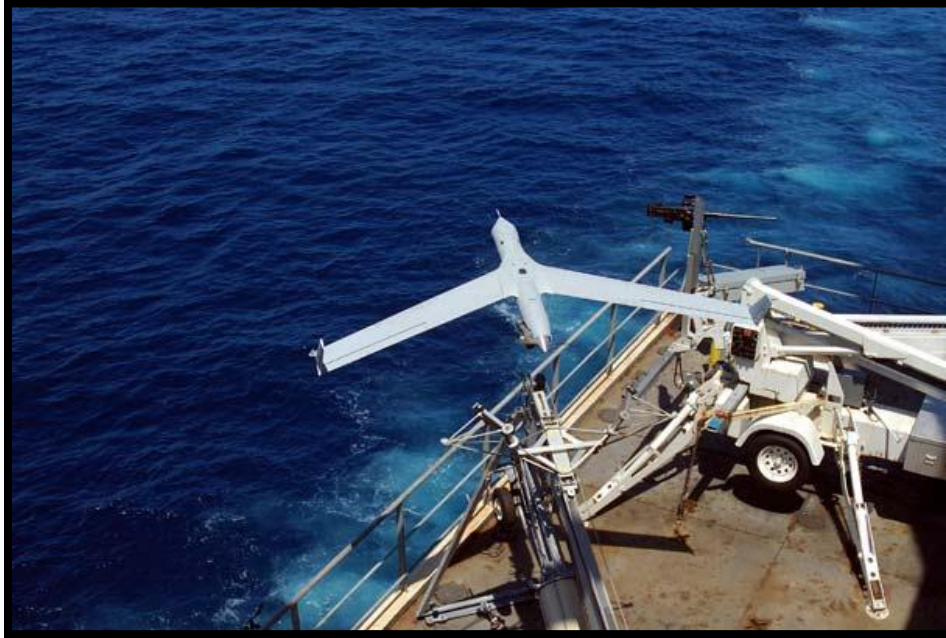
Figure 3–1. Boeing-Insitu ScanEagle taking flight from launcher onboard a ship.
