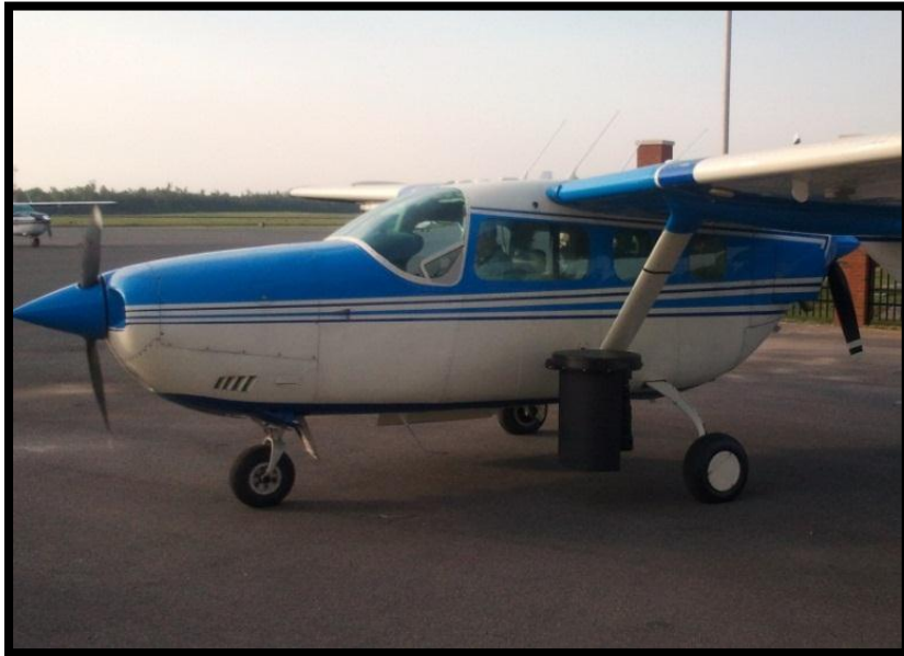
Figure 3–2. Cessna 337 Skymaster with side mounted camera system.
