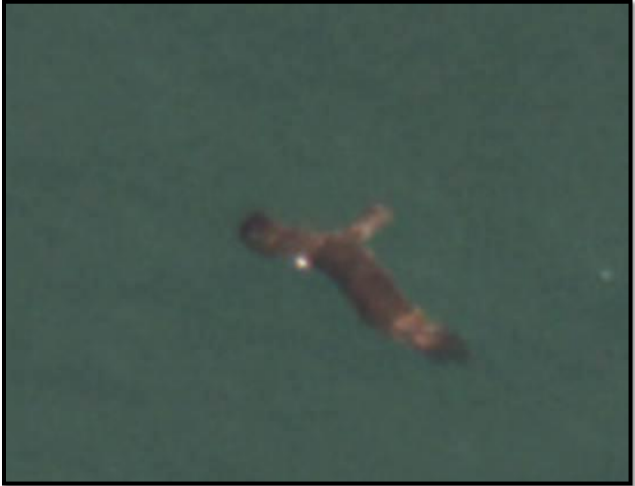
Figure 3–10. Osprey ( Pandion haliaetus )—Image captured by a gyrostabilized high-resolution area-scan camera mounted externally to a Cessna 337 Skymaster aircraft during experimental imaging flights conducted by the project team 10 to 20 May 2011 offshore of Oak Island NC. This image has a resolution of 1.5 cm and was taken from a survey flight altitude of 433 m.
