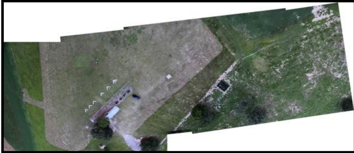
Figure 2–23. Composite image of the ground surface near Gainesville FL, created by stitching together four separate images taken during stage 2 flight testing of the imaging system developed for UAS-based deployment, September 2011.
