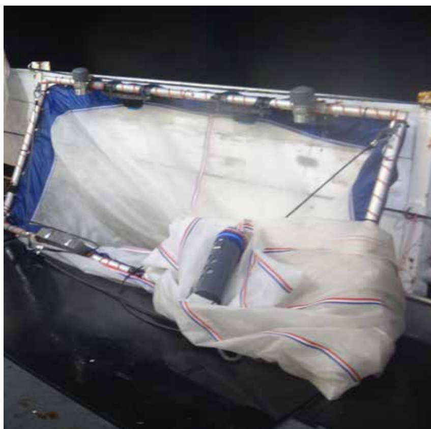
Figure 10-4 Photograph of Go-Pro cameras and lights deployed on the top bar of the frame-net From the 2017 NOAA ship Henry B. Bigelow cruise HB1704.
