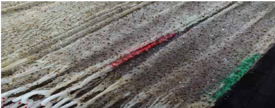
Figure 10-3 Photograph of clogging the mesh of the midwater trawl
