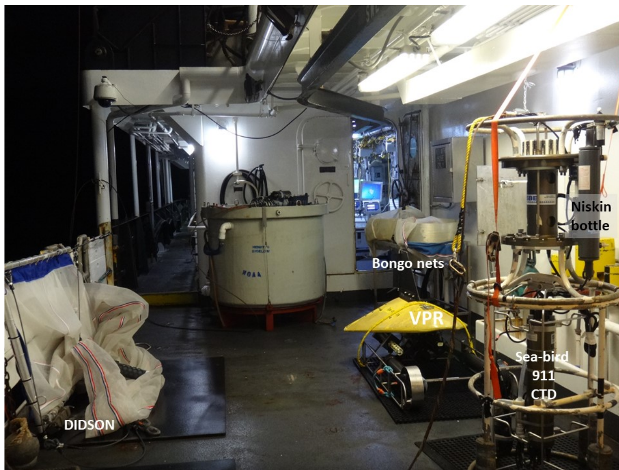
Figure 10-7 Sea-bird 911 CTD on a 12 Niskin bottle rosette
