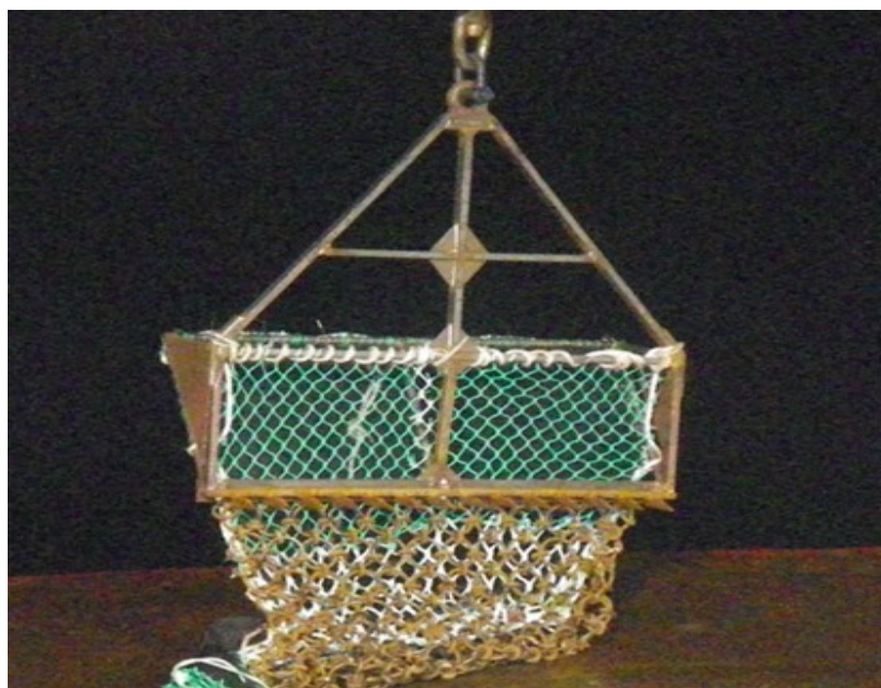
Figure 5.2 Modified 1.24m shellfish (sandeel) dredge
