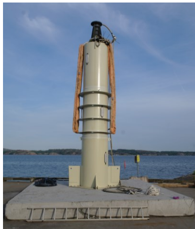
Figure 2. Uppsala University linear Wave Energy Converter (WEC) on foundation, without buoy, onshore before deployment.
