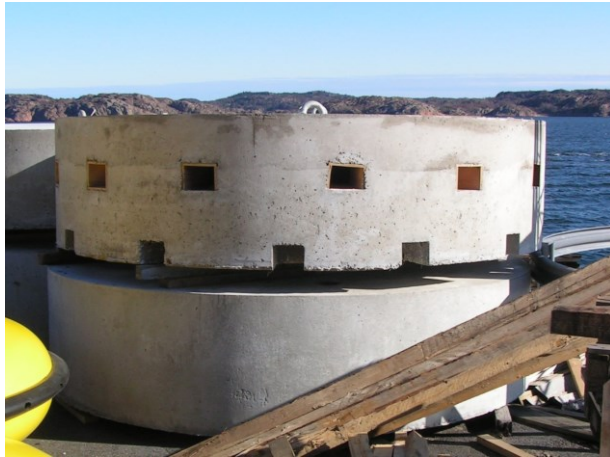
Figure 4. Two ecological foundations for environmental and ecological studies in the Lysekil research site. The upper ecological foundation includes manufactured holes for increased complexity, and the lower foundation resembles a non-complex foundation.
