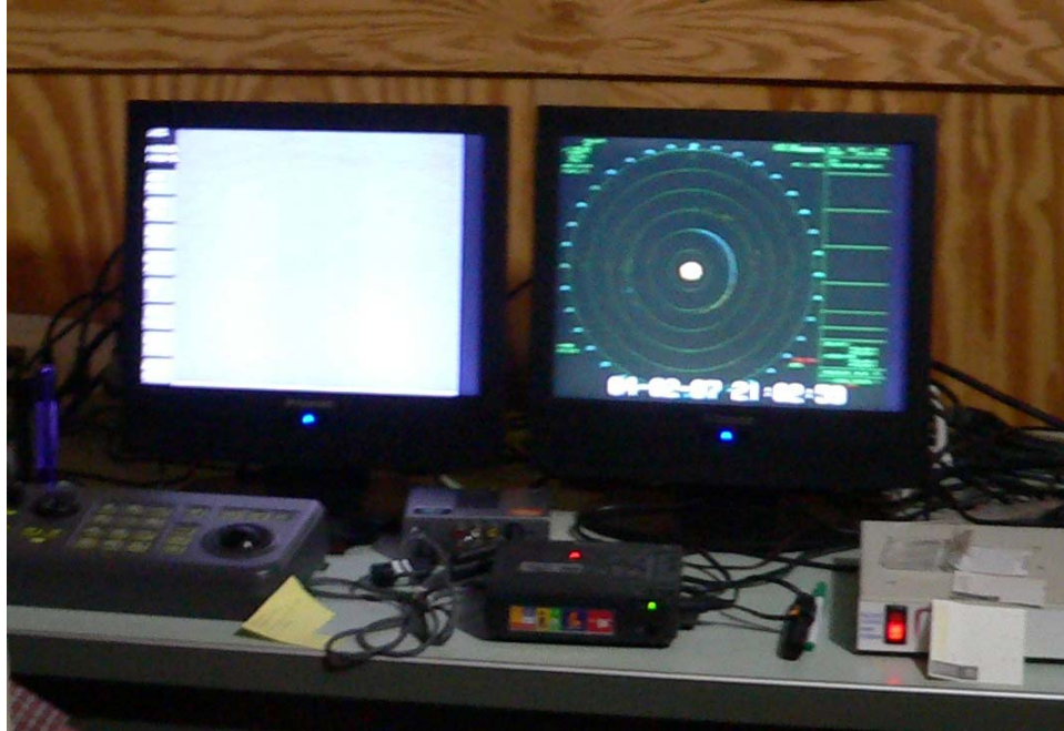
Figure 6-9. Dual display of video from thermal imager (left) and vertically-pointing radar (right).
