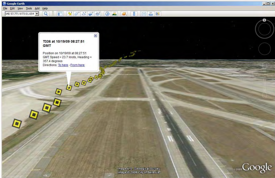
Figure 6-76. An individual track exported to kml format and viewed in Google Earth.
