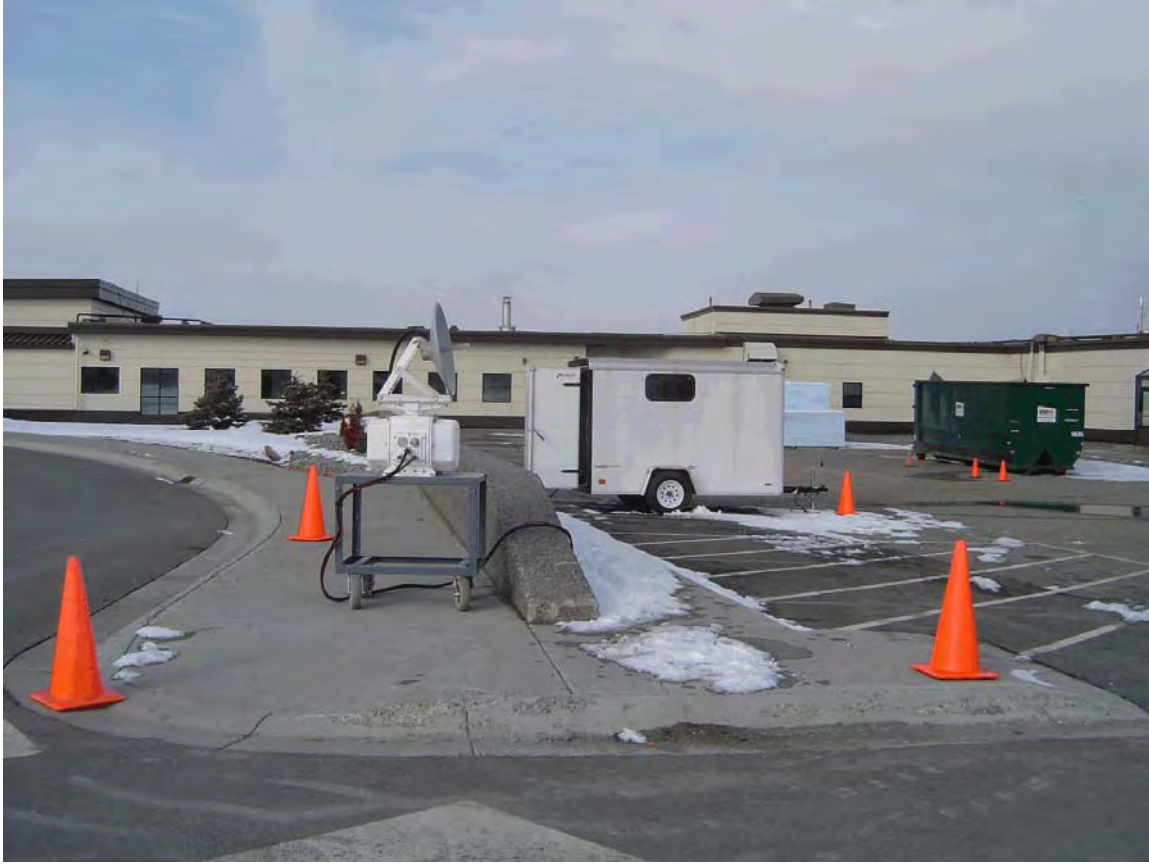
Figure 6-126. eBirdRad unit at Elmendorf Air Force Base in April 2008, prior to mounting the transceiver on the roof of the Operations Building in the background.
