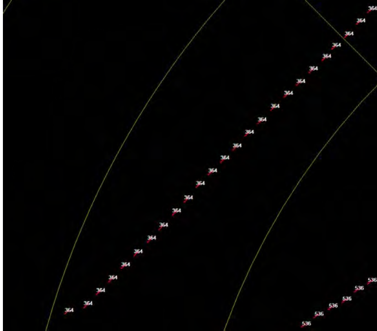
Figure 6-113: TVW display showing tracks from the WIAR1 radar at NASWI on 13 November 2009. The Track ID (only the three least significant digits) is shown at each track update. The Track ID of interest is 364.
