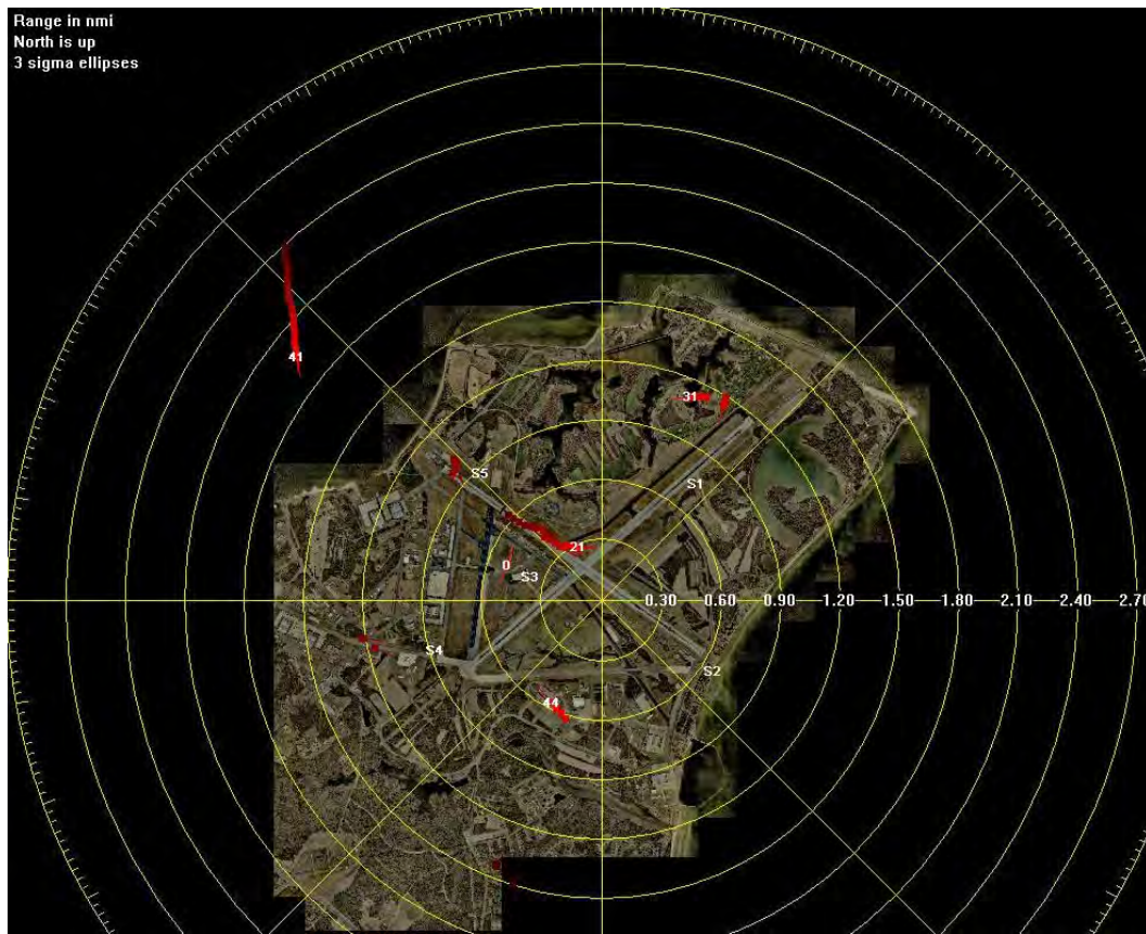
Figure 2-6. Typical display of eBirdRad avian radar system, NAS Patuxent River, 17 April 2007, 21:45 EDT. North is up; radar range setting is 3 nmi (5.5 km), range rings are 0.3 nmi (556 m) apart. Red trails are target tracks; white label at the head of a track is the target's speed, in knots.
