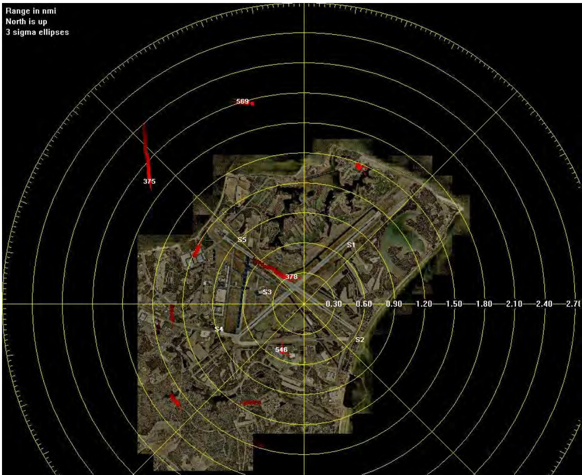
Figure 6-42. eBirdRad display based on the same data as Figure 6-41, with true trail mode turned off and automatic tracking and track history turned on. The red trails are the positions (“history”) of the target while it was being tracked; the white label at the head of a track is the target’s Track ID.
