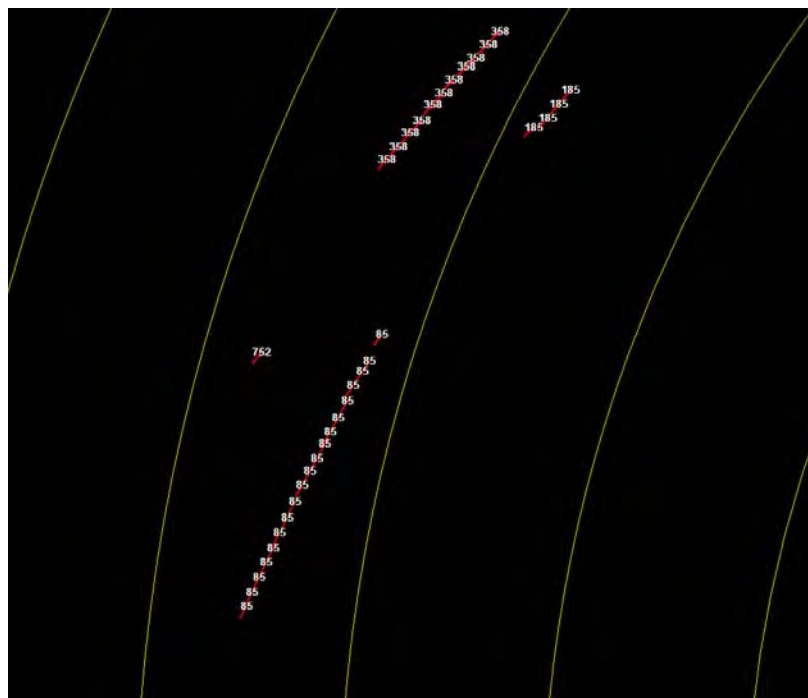
Figure 6-109: TVW display showing tracks from the WIAR1 radar at NASWI on 13 November 2009. The Track ID (only the three least significant digits) of each target is shown for each track update.
