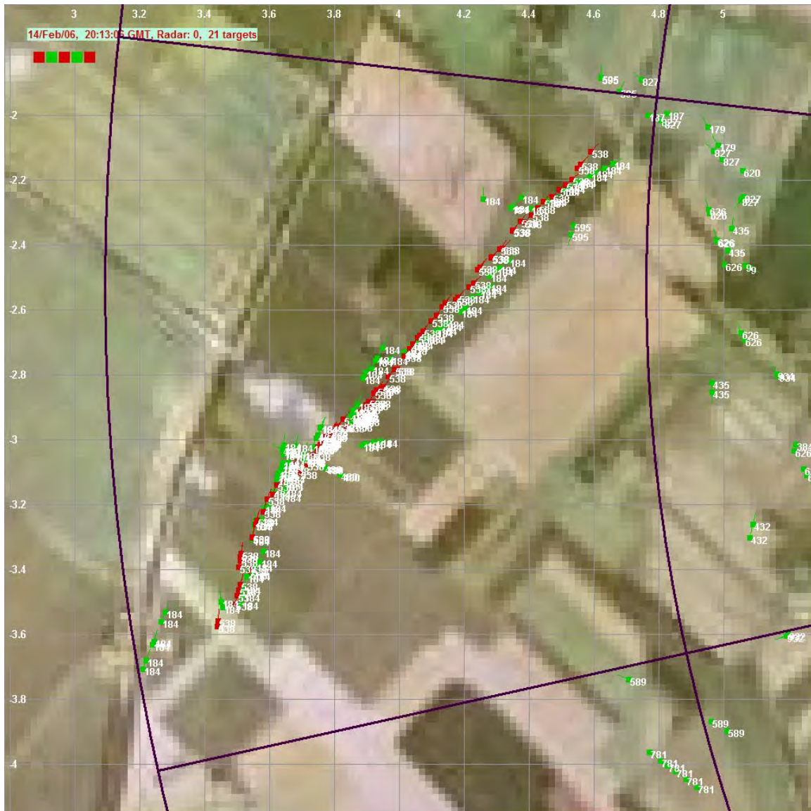
Figure 6-118: Zoomed region of interest from two MCASCP radars deployed to a site in Washington County, North Carolina, on 14 February 2006, showing tracks from the respective radars with the Track IDs displayed. No fusion processing was applied. Green Track ID 184 (from eastern radar) and red Track ID 538 (from western radar) are long tracks.
