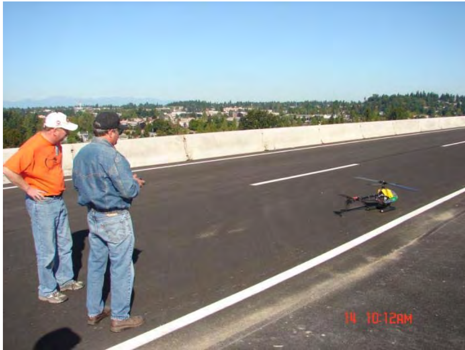
Figure 6-14. Remote-controlled helicopter (RCH) on the SEA perimeter road with pilot and observer.
