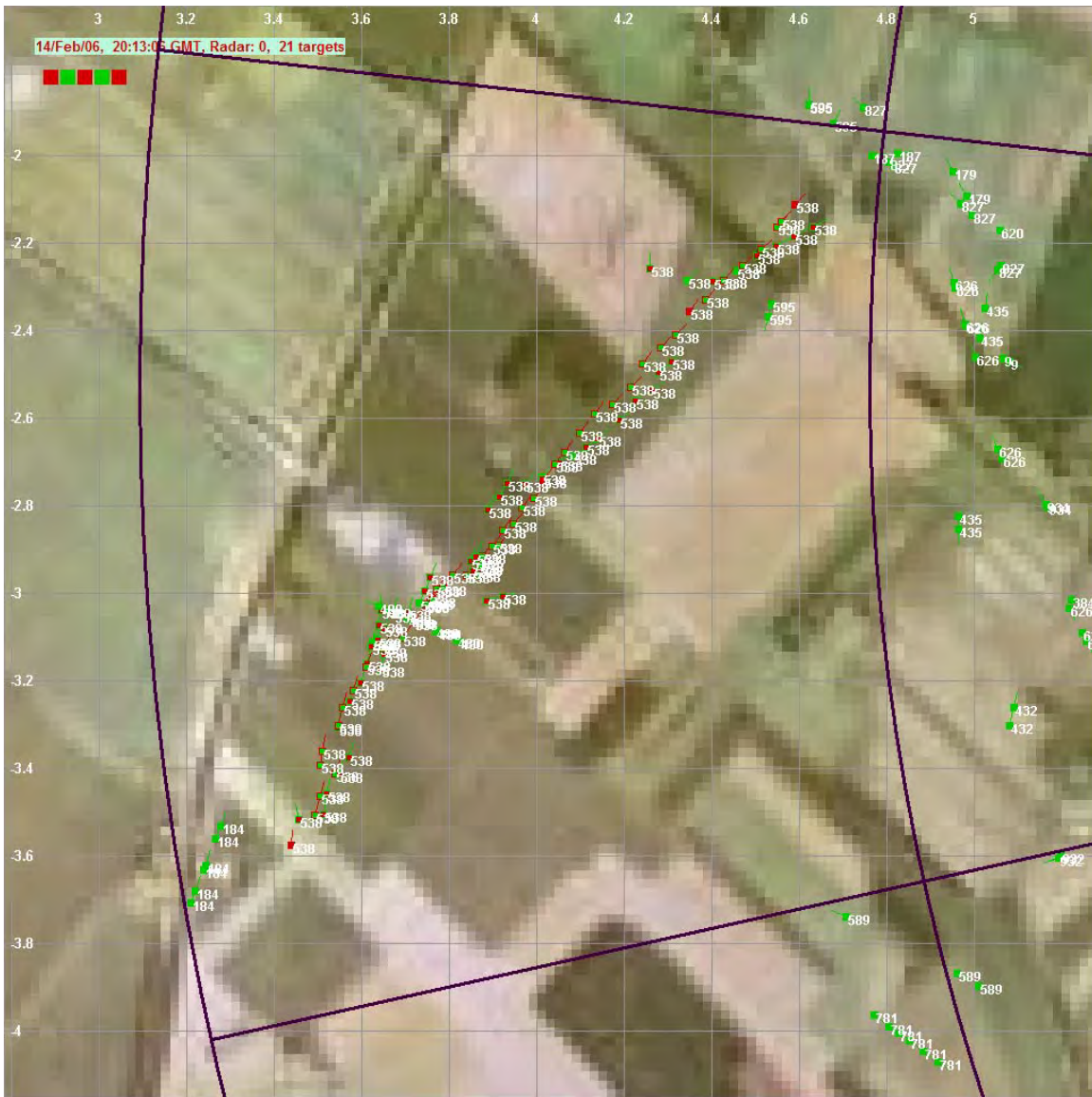
Figure 6-119: Region of interest from two MCASCP radars deployed to a site in Washington County, North Carolina, on 14 February 2006, after fusion processing. Green Track ID 184 from the eastern radar and red Track ID 538 from the western radar have been combined into fused Track ID 538.
