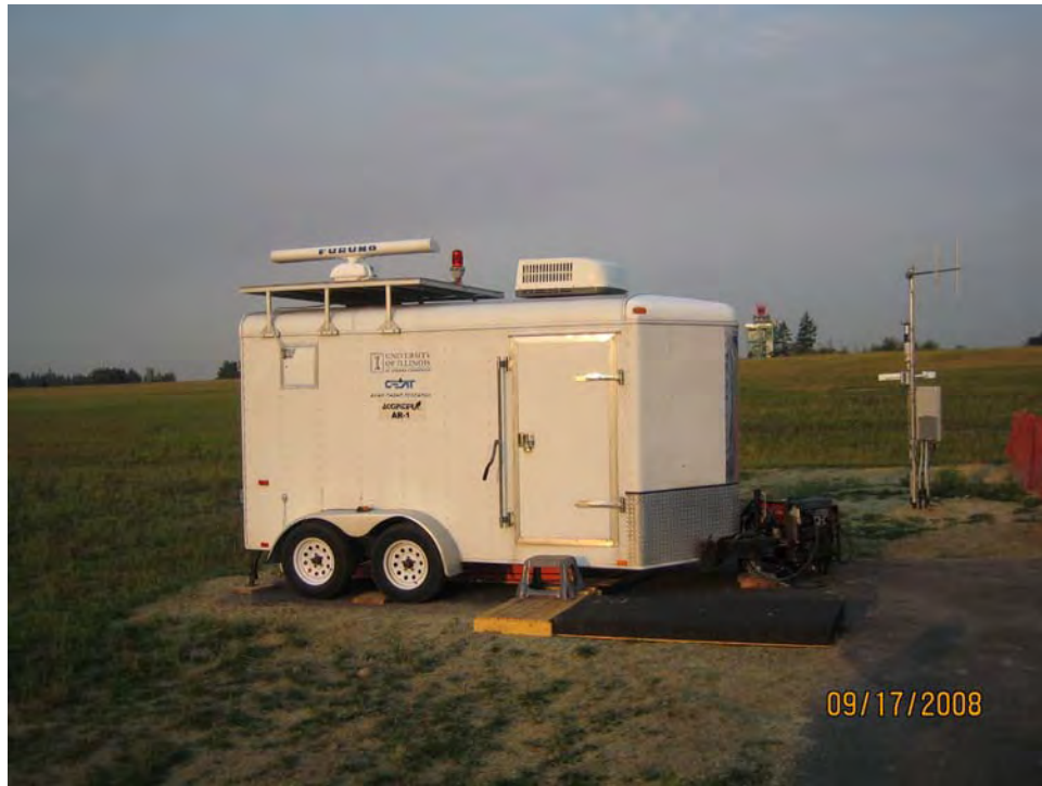
Figure 2-10. AR-1 (SEAAR1m) array antenna system located at SEA. The Port of Seattle station that provides power and the ASR radar for SEA is in the background.
