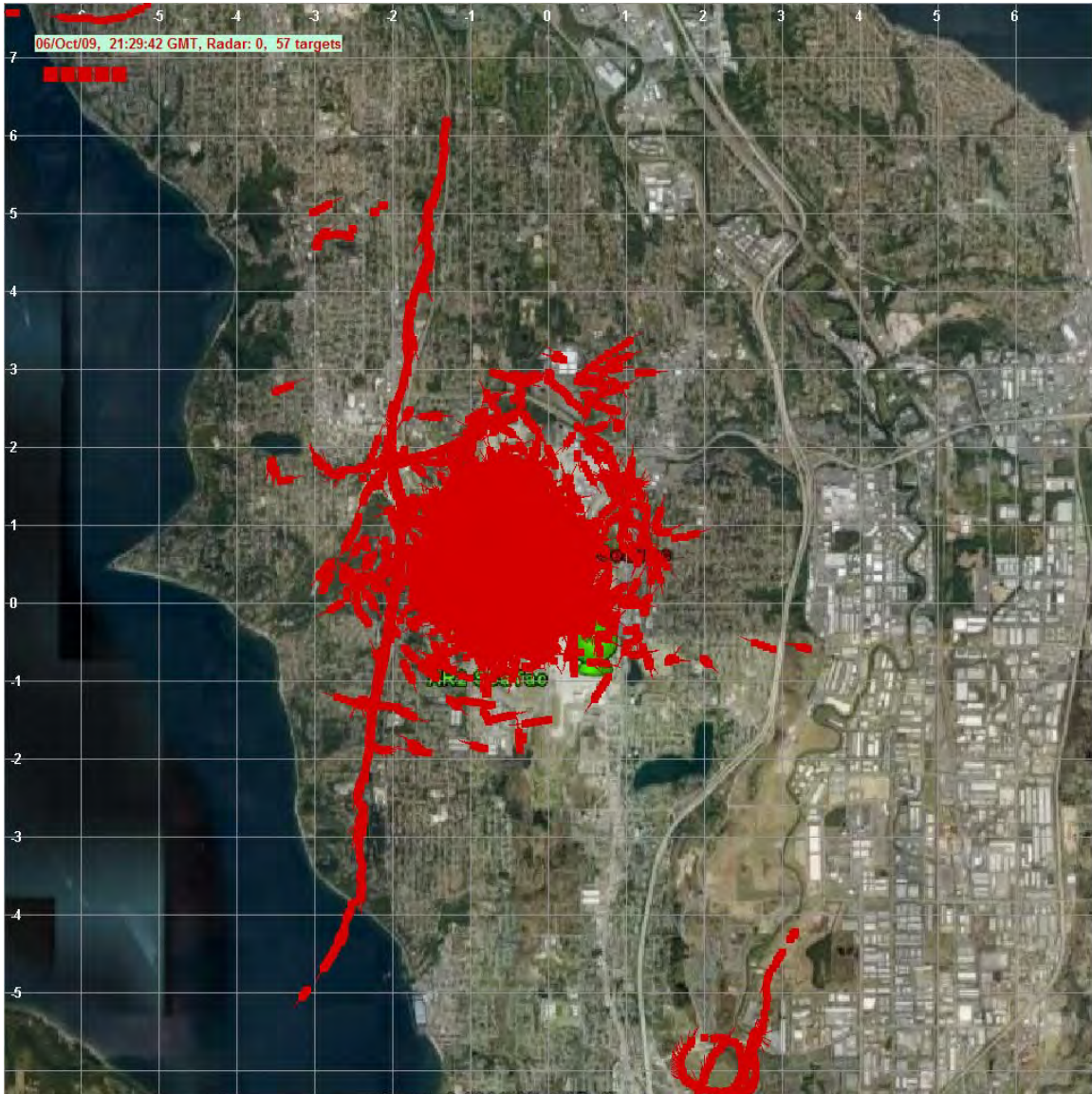
Figure 6-120: SEA SEAAR1m radar tracks over the 13 minute interval of interest on 06 October 2009. The long track extending from about 6 km north to about 5 km south is the flock of interest. The speed of individual tracks in this flock is about 15 m/s. The SEAAR1m radar has good coverage to the west of the airfield because the radar is in a bowl below runway grade, and hence has a natural clutter fence.
