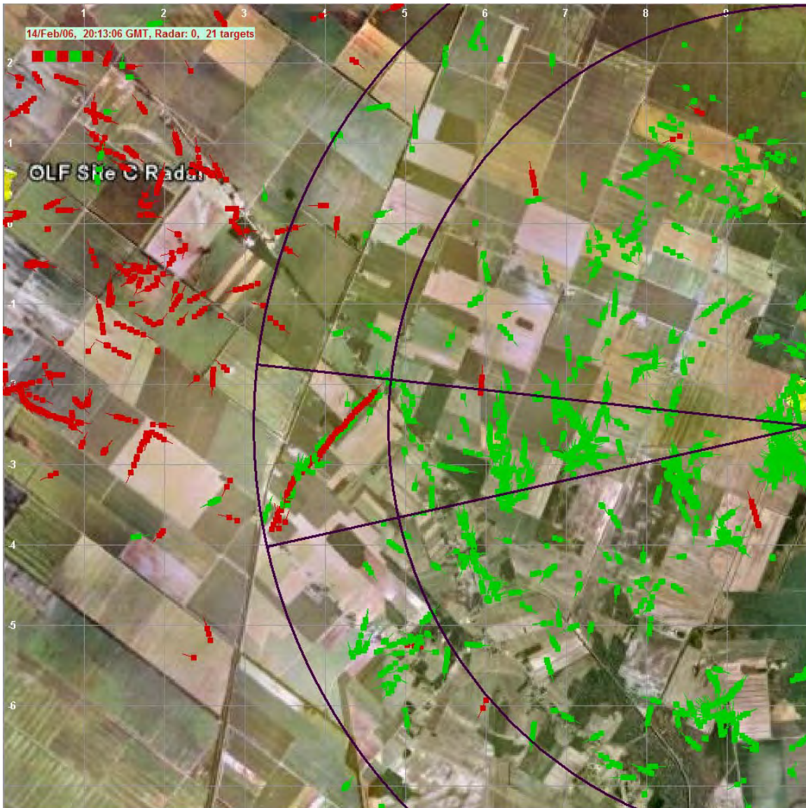
Figure 6-117: Integrated tracks (no fusion) from two MCASCP radars deployed to a site in Washington County, North Carolina, on 14 February 2006. The red tracks were generated by the western radar (yellow pushpin near the top-left of the display); the green tracks were generated by the eastern radar (pushpin at the extreme right, midway up the display). These two radars are over 10 km apart. The tracks of interest are those in the overlapped region shown near the middle of the display, contained within the range-azimuth region bounded by the circular range markers and the radial electronic bearing lines. Each gray grid cell in this figure represents a 1 km by 1 km square.
