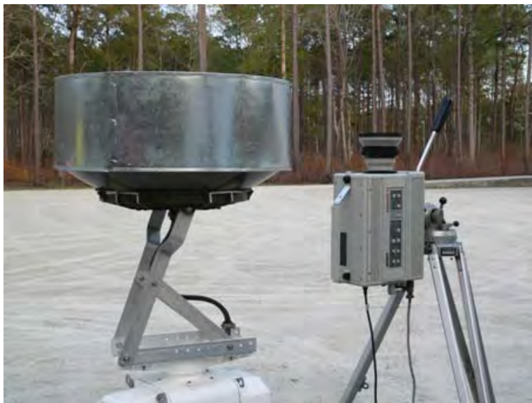
Figure B-10. The TI-VPR sensors: A Furuno FR2155-BB 50 kW X-band radar with a vertically-pointing parabolic dish (left), and Radiance I high-resolution thermal imaging camera (right).
