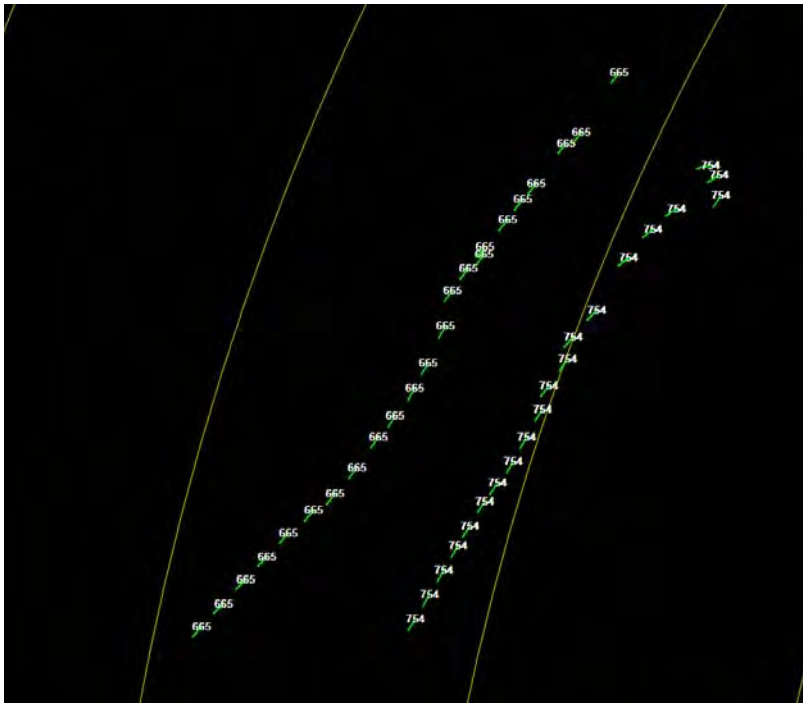
Figure 6-110: TVW display showing tracks from the eBirdRad radar at NASWI on 13 November 2009. The Track ID (only the three least significant digits) of each target is shown for each track update.
