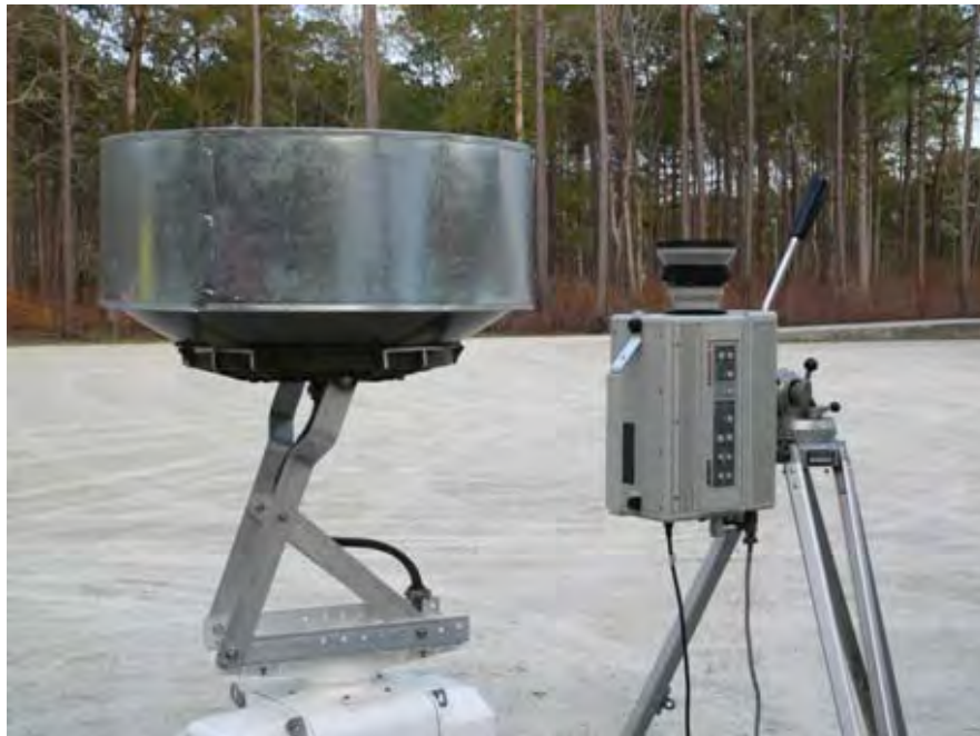
Figure 6-4. The basic sensor elements of the TI-VPR, including a 50 kW X-band Furuno model FR2155-BB radar with a vertically-pointing 4° parabolic dish antenna (left), and Radiance I high-resolution thermal imaging camera (right).
