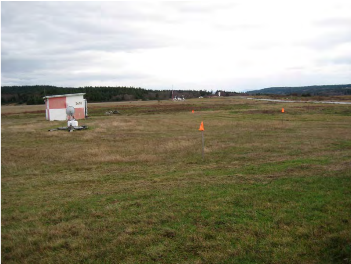
Figure 6-125. eBirdRad avian radar at NAS Whidbey Island, showing orange safety cones used to indicate to personnel the safe distance to approach the radar when it is operating.
