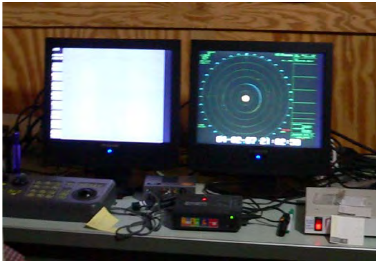
Figure B-14. Dual display of video from thermal imager (left) and vertically-pointing radar (right).
