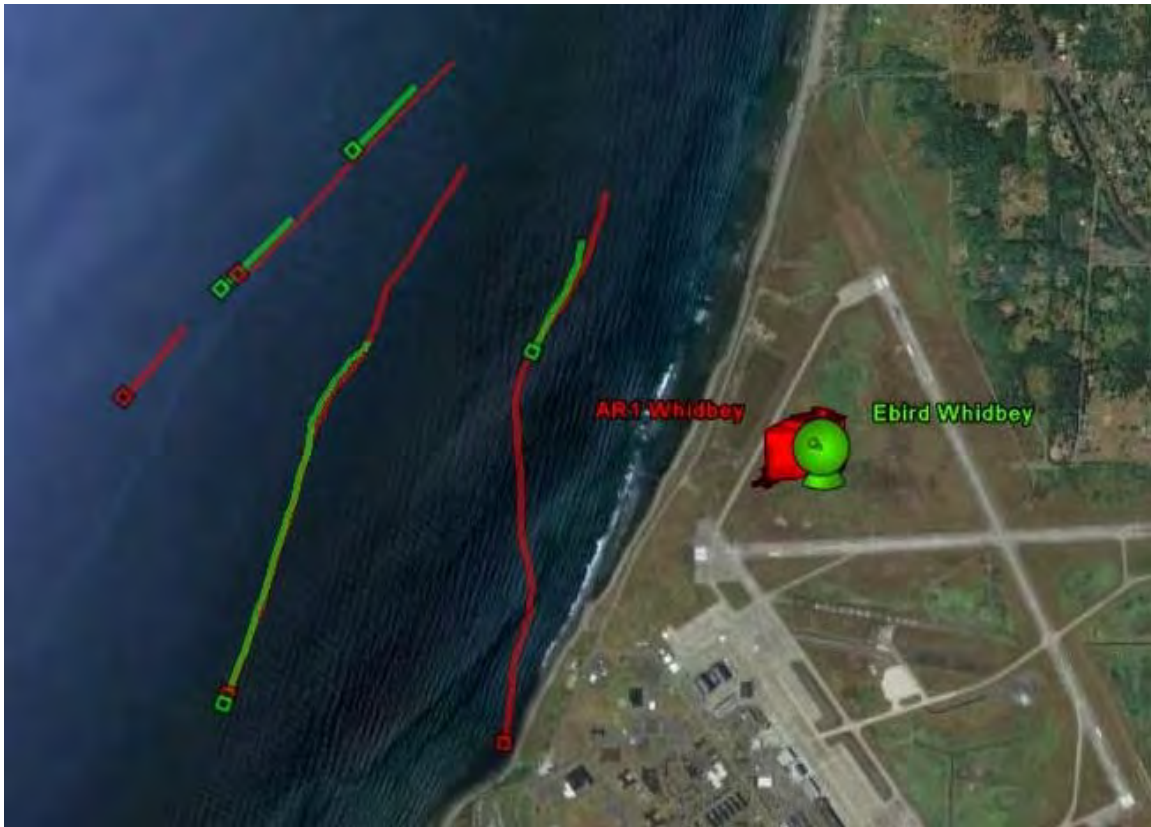
Figure 6-105. Track histories of targets selected from WIAR1 and WeBirdRad radars at WASNI dataset for spatial alignment analysis. The green symbols represent the WeBirdRad unit and the red the WIAR1.
