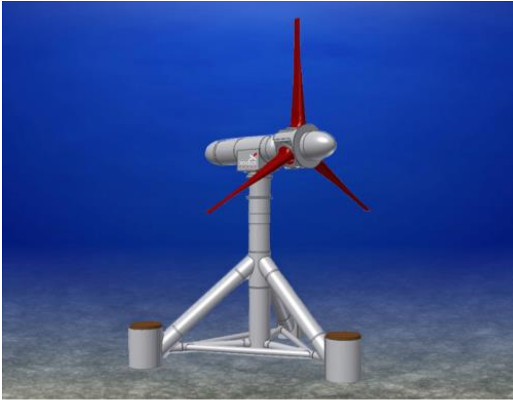
Figure 5.5: Typical horizontal axis turbine (Xodus.com)
