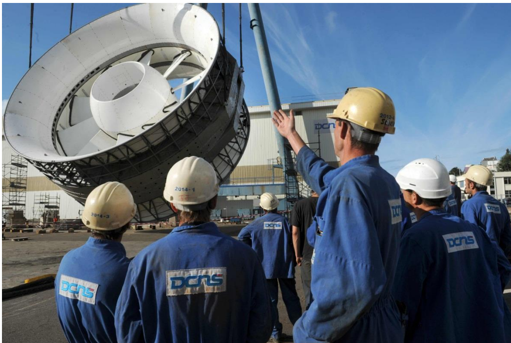
Figure 1.2: 16m Open-Centre Turbine, France
