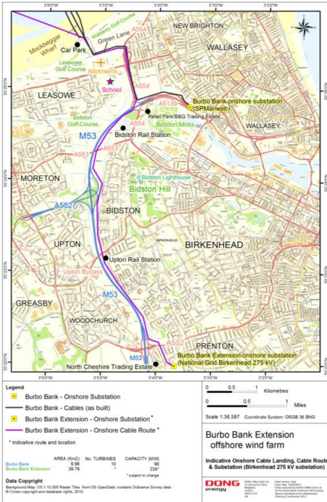
Chart 4: The Burbo Bank Extension indicative onshore cable landing, cable route and onshore substation at the National Grid Birkenhead 275 kV substation
