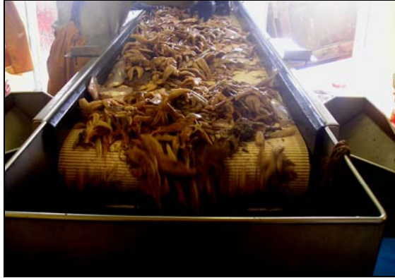
Figure 3. Conveyor and chute in the whale-back of 'Admiral Grenville'
