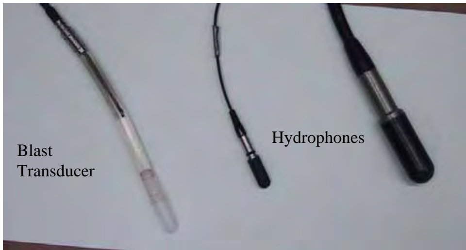
Figure II-5. Example of Different Pressure Sensors
