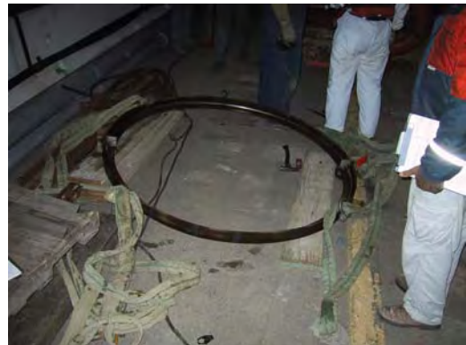
Figure I.10-6 Simple Air Bubble Curtain System Used To Attenuate Sounds for 30-Inch-Diameter Piles
