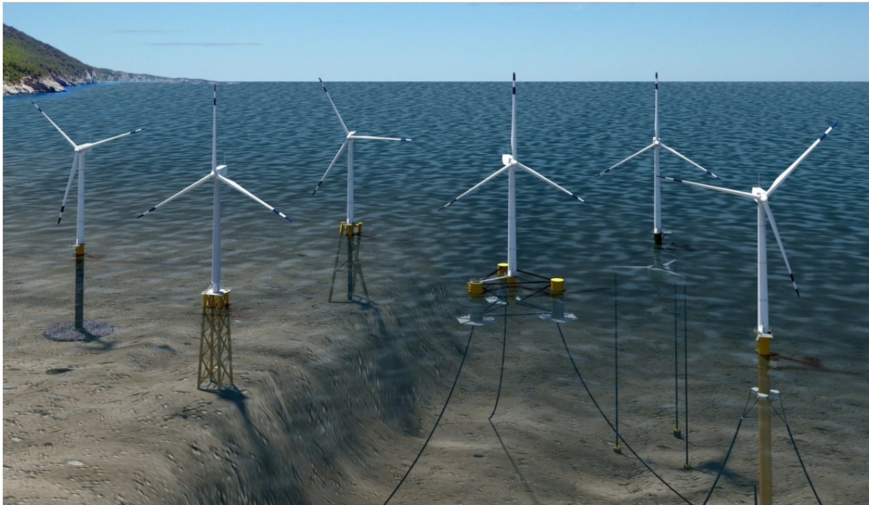
Figure 1: Offshore wind foundation types
