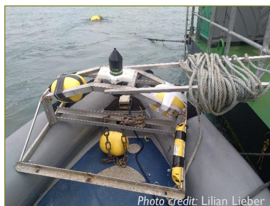
Figure 10. VEMCO V9 HR Range Test Tags (left) and custom-made bracket and frame for seabed deployment. Deployment notes: Frame modified by Aidan Flaherty, Queen's University Belfast (QUB) and Joel Hoy, Minesto. Receiver bracket manufactured by Aidan Flaherty (QUB). Tag brackets for deployment onto barge/mooring chains manufactured by Joel Hoy.
